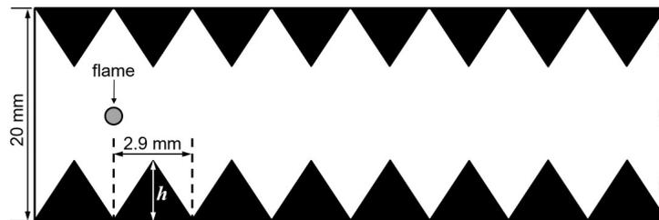
Figure 1. Computational domain of a channel with triangular obstacles. Adiabatic, reflecting and no-slip boundary conditions are applied for the walls and obstacle surfaces. Four obstacle heights  $h = 1, 3, 5$ , and  $7$  mm are used, corresponding to blockage ratio  $br = 0.1, 0.3, 0.5$ , and  $0.7$ , respectively. Initial flame radius is 1 mm.
