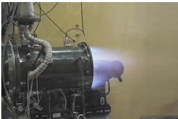
Fig.5. Typical picture of the flame emerging from rotating detonation chamber.
