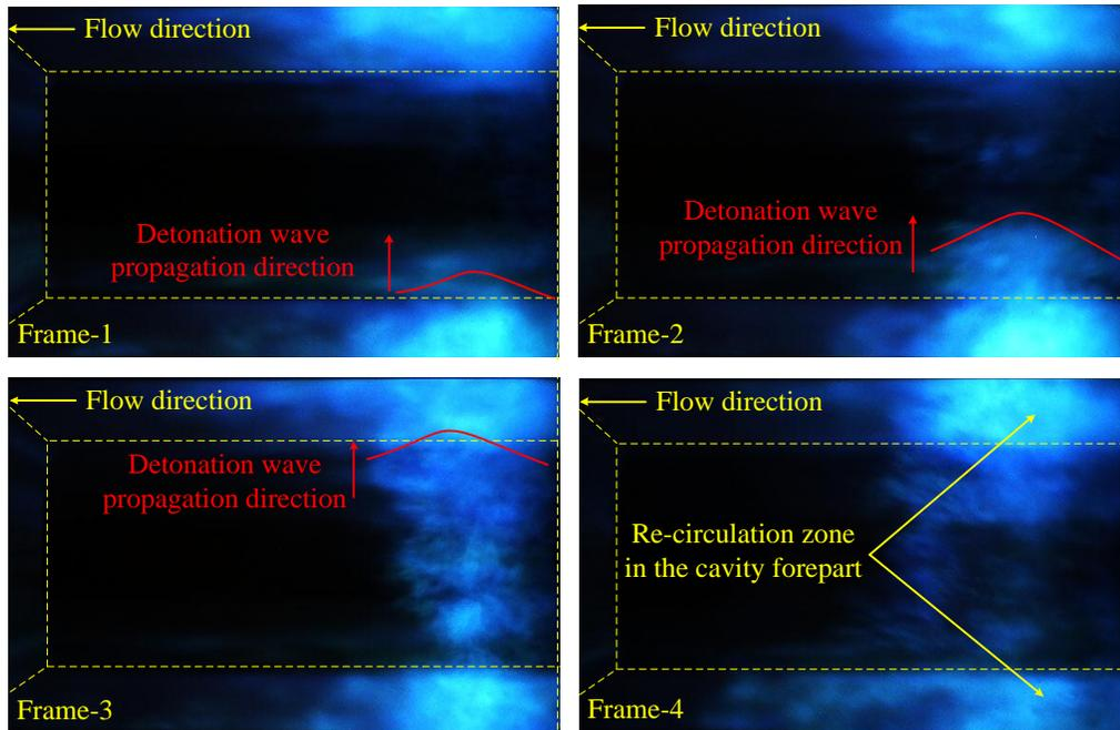
Fig.4 High-speed photography images of two-waves in homo-rotating mode in Test #1
