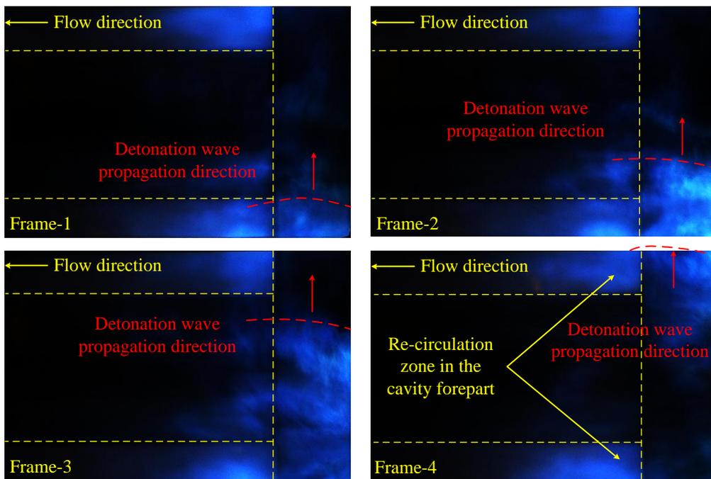
Fig.5 High-speed photography images of two-waves in homo-rotating mode in Test #2
