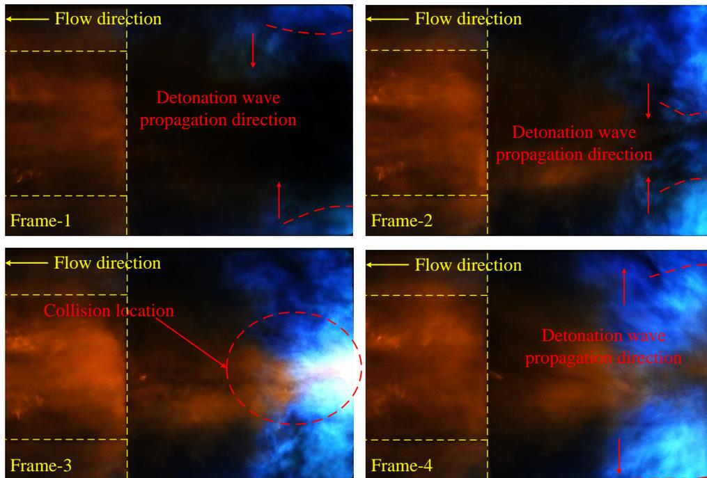
Fig.7 High-speed photography images of two-waves in hetero-rotating mode in Test #4
