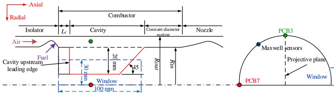
Fig.1 Schematic diagram of the annular combustor with cavity
