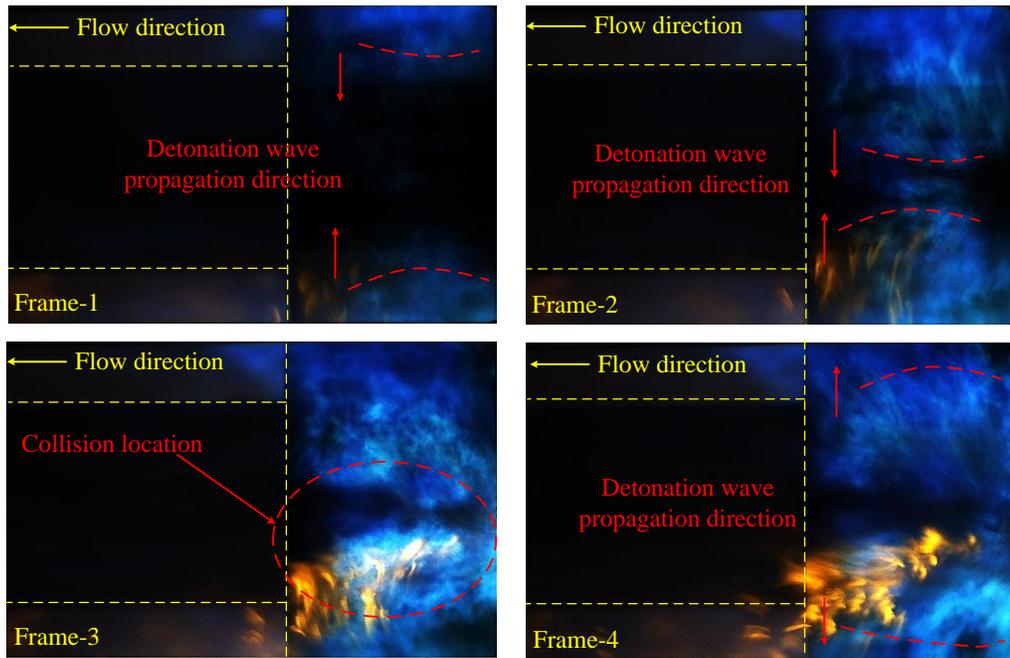
Fig.6 High-speed photography images of two-waves in hetero-rotating mode in Test #3
