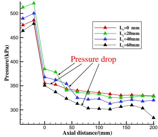
Fig.3 Axial pressure distribution
