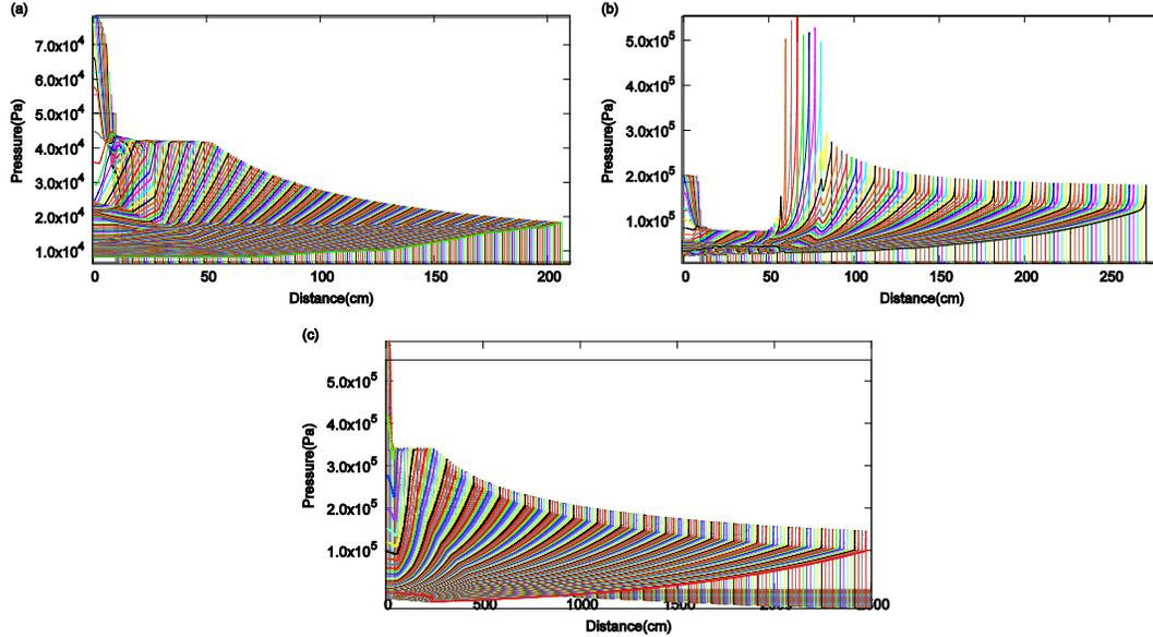
Figure 3. Different regimes of detonation initiation with  $r_s=10$  cm and  $T_s=1800$  K, (a) subcritical case ( $p_s=50$  kPa), (b) critical case ( $p_s=122$  kPa), (c) supercritical case ( $p_s=2000$  kPa)
