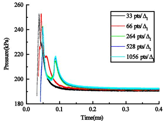
Figure 2. Pressure of the shock front in different resolutions
