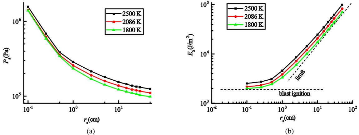
Figure 5. Critical pressure and critical internal energy for the detonation ignition, (a) critical pressure, (b) critical internal energy
