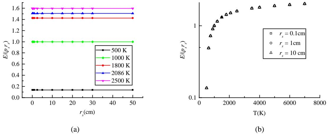
Figure 6. Non-dimensional critical internal energy in the energy source, (a) as a function of  $r_s$ , (b) as a function of  $T$
