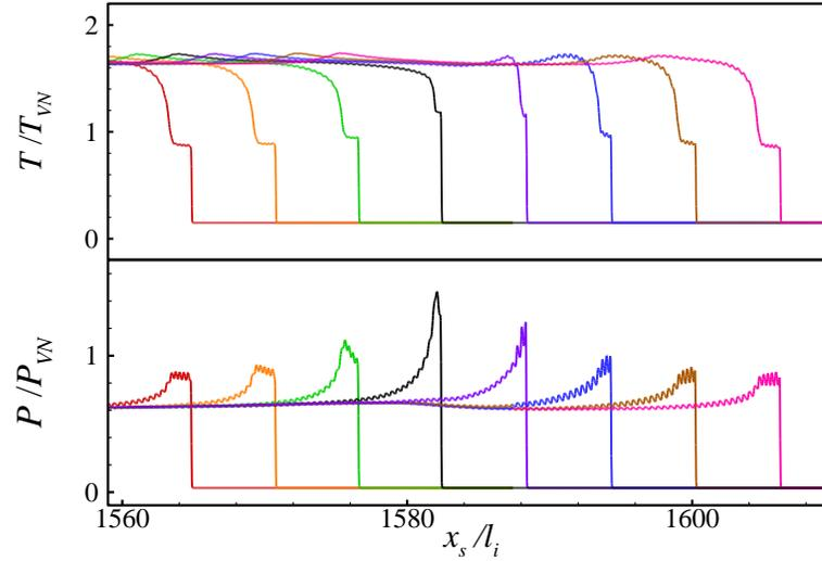
Fig. 5 Evolution of detonation structure for the case with  $400\pi$  during  $t = 22.266, 22.392, 22.514, 22.625, 22.727, 22.842, 22.965, 23.092 \mu\text{s}$ .
