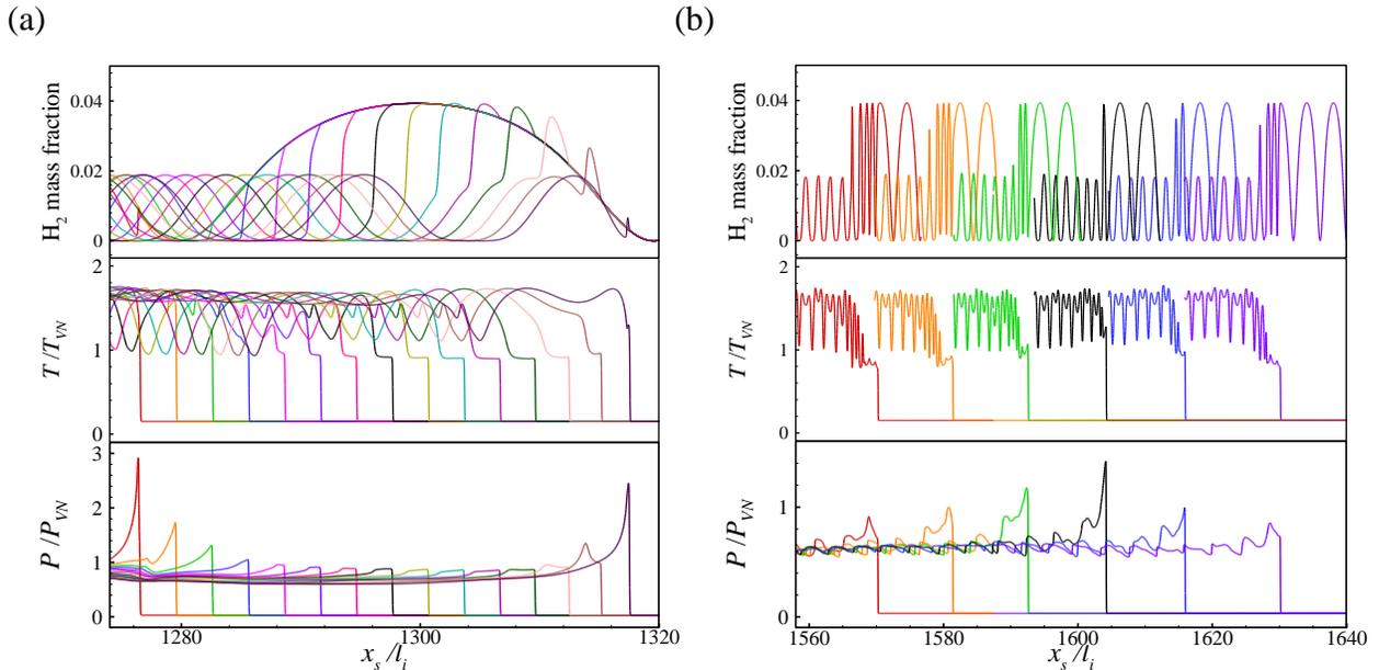
Fig. 4 Evolution of detonation structure for  $4\pi$  and  $40\pi$ : (a)  $t = 23.665, 23.712, 23.768, 23.828, 23.888, 23.948, 24.006, 24.064, 24.123, 24.181, 24.240, 24.299, 24.358, 24.415, 24.465 \mu\text{s}$ ; (b)  $t = 22.878, 23.124, 23.358, 23.572, 23.795, 24.097 \mu\text{s}$ .
