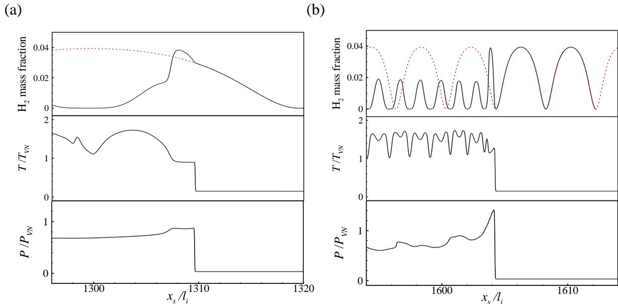
Fig. 3 Detonation front structures for frequencies of  $4\pi$  (a) and  $40\pi$  (b): red dash line is initial gradient.
