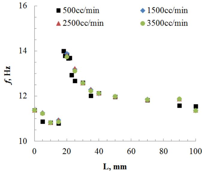
Fig. 3 Effect of burner separation distance on flickering frequency for varying of fuel flowrate. All cases shown here are at burner diameter of 10.8 mm
