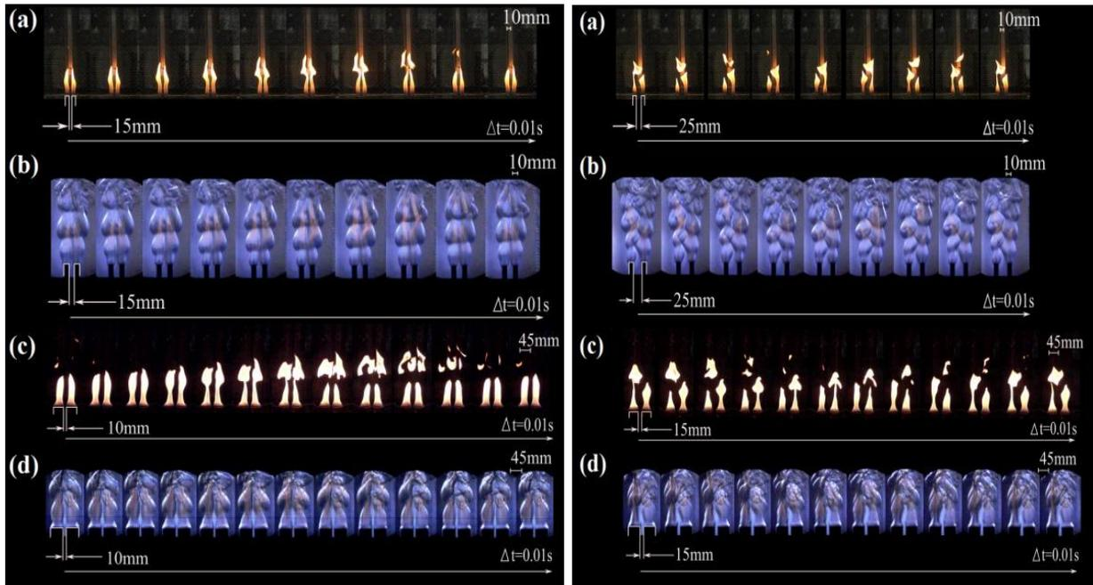
Fig. 2 Instantaneous image-sequence of pulsating methane plume and schlieren imaging under in-phase (left) and anti-phase (right) modes (a-b:  $d = 10.8$  mm,  $L = 15$  mm (left),  $L = 25$  mm (right),  $Re = 76$ ,  $Q = 1000$  cc/min; c-d:  $d = 45$  mm,  $L = 10$  mm (left),  $L = 15$  mm (right),  $Re = 37$ ,  $Q = 2000$  cc/min; Time interval: 0.01s)
