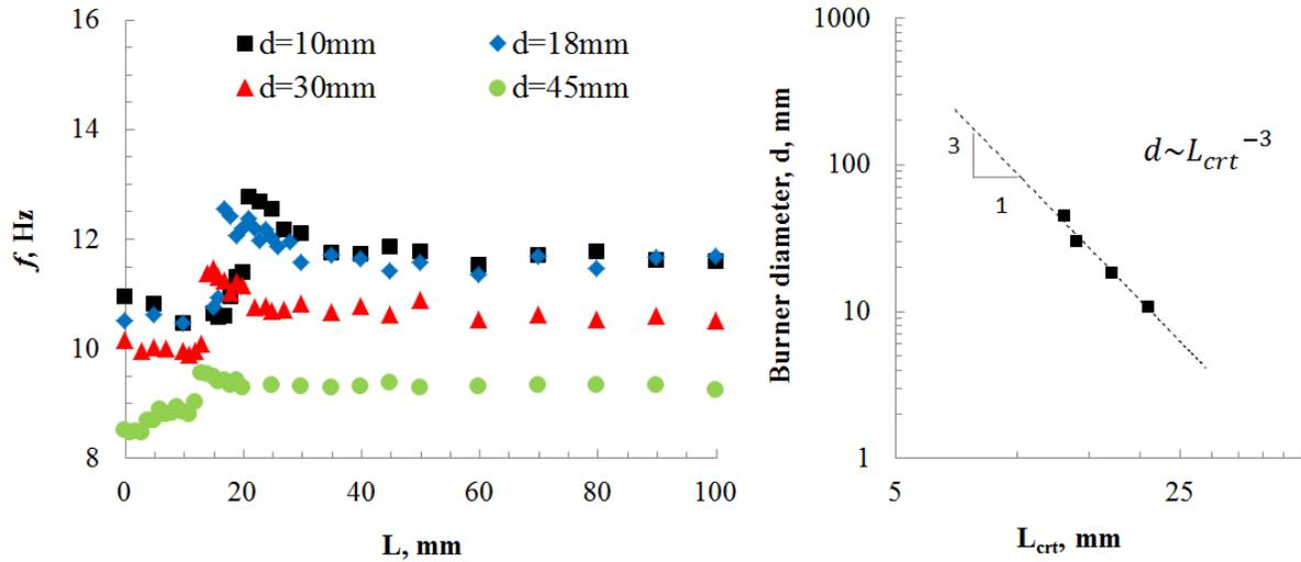
Fig. 4 Effect of burner separation distance on flickering frequency for various burner diameters (left) and dependency of critical separation distance ( $L_{crt}$ ) on burner diameter  $d$ . All cases shown here are at fuel flowrate of 1000 cc/min except for 45 mm of 2000 cc/min
