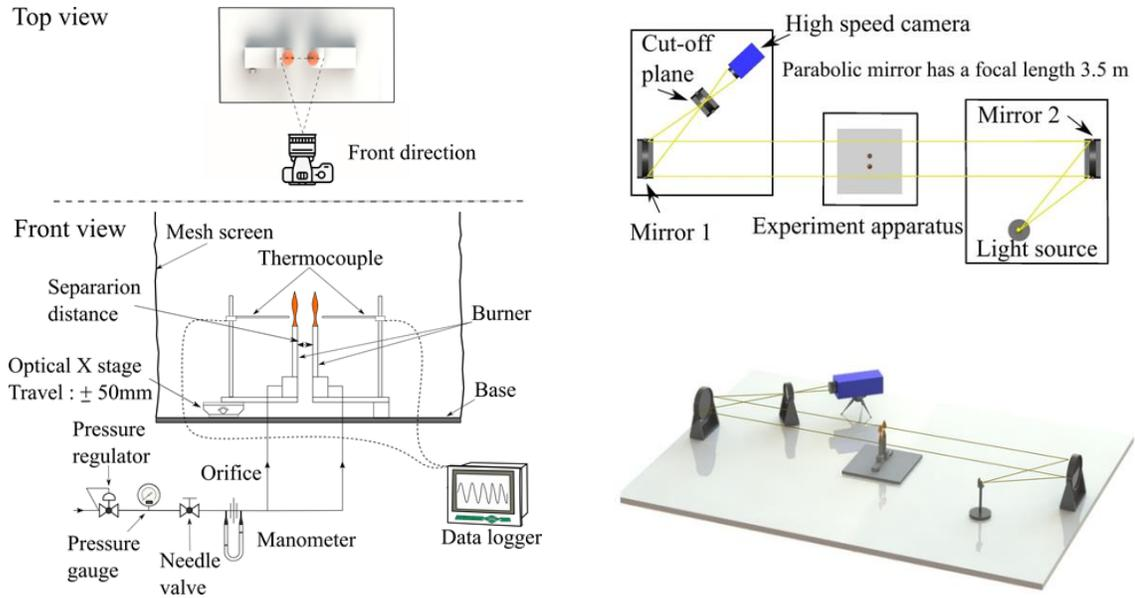
Fig.1 Schematics of experimental apparatus.
