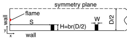
Figure 1: Computational setup.  $D = 0.174$  m,  $H = 2.61 \times 10^{-2}$  m,  $S = 0.174$  m,  $W = 2 \times 10^{-2}$  m,  $L = 11.878$  m. Blockage ratio  $br = 0.3$ . Initial flame radius is  $2.5 \times 10^{-3}$  m.
