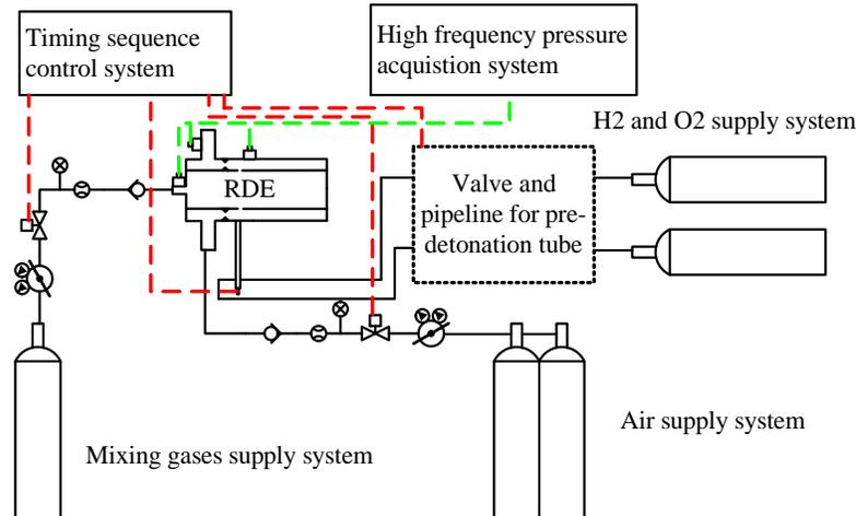
Fig 1 Sketch of the experimental system
