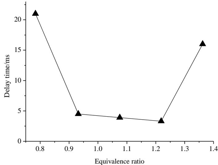
Fig 5 Delay time of rotaing detonation with different equivalence ratios
