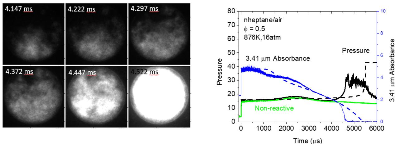
Fig. 1. Near-homogeneous ignition in the HPST; n-heptane/air,  $\phi = 0.5$ ,  $T = 876$  K,  $P = 16.0$  atm. Dashed lines are simulated fuel and pressure time histories using the Lawrence Livermore National Laboratory (LLNL) gasoline surrogate detailed mechanism and a constant volume Chemkin model [1].
