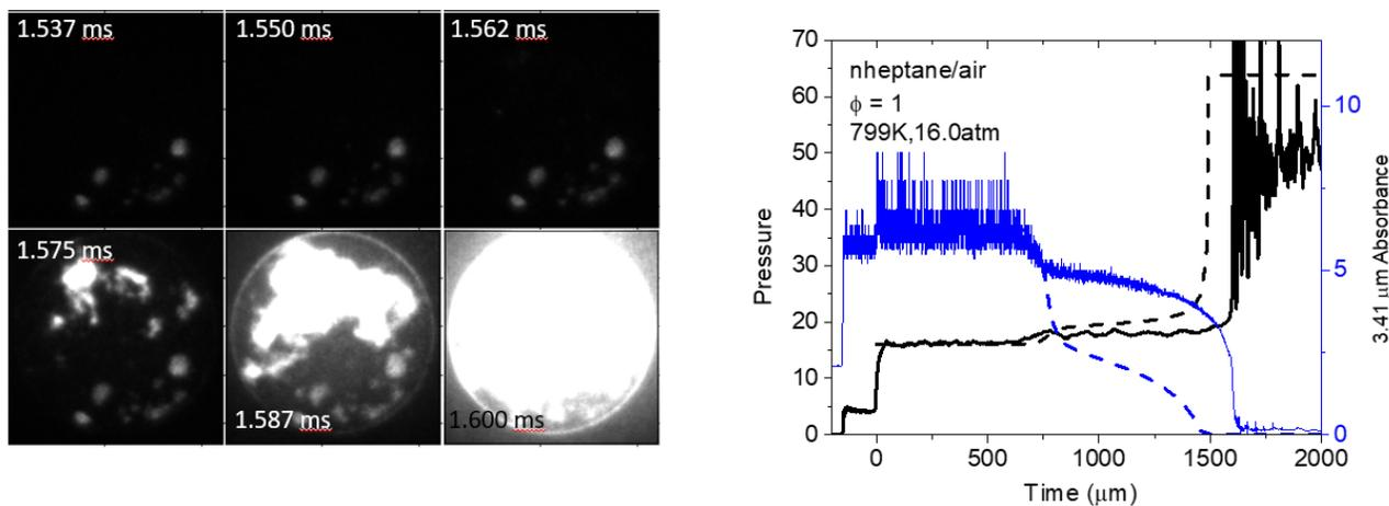
Fig. 2. Near-homogeneous ignition in the HPST; n-heptane/air,  $\phi=1$ ,  $T=799$  K,  $P=16.0$  atm. Dashed lines are simulated fuel and pressure time histories using the Lawrence Livermore National Laboratory (LLNL) gasoline surrogate detailed mechanism and a constant volume Chemkin model [1].
