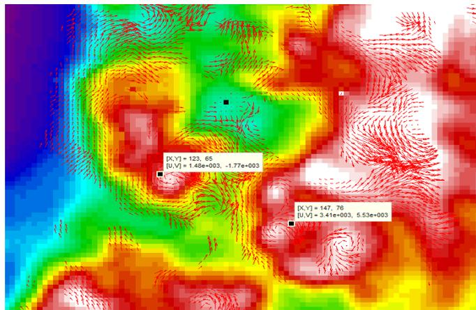
Figure 6. Expending gases velocity and direction
