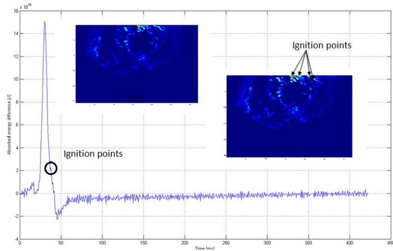
Figure 4. Explosion ignition point propagation graph
