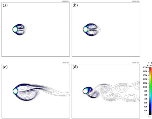
Figure 5 The transient evolution of vortex shedding in terms of temperature for case #3 : (a)  $t = 2 \times 10^{-3}$  sec; (b)  $t = 3 \times 10^{-3}$  sec; (c)  $t = 1 \times 10^{-2}$  sec; (d)  $t = 5 \times 10^{-2}$  sec
