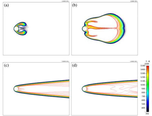
Figure 6 The transient evolution of vortex shedding in terms of temperature for case #4 : (a)  $t = 2 \times 10^{-3}$  sec; (b)  $t = 3 \times 10^{-3}$  sec; (c)  $t = 1 \times 10^{-2}$  sec; (d)  $t = 5 \times 10^{-2}$  sec
