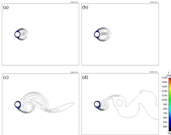
Figure 3 The transient evolution of vortex shedding in terms of temperature for case #1 : (a)  $t = 2 \times 10^{-3}$  sec; (b)  $t = 3 \times 10^{-3}$  sec; (c)  $t = 1 \times 10^{-2}$  sec; (d)  $t = 5 \times 10^{-2}$  sec
