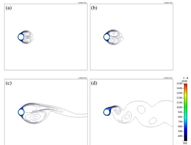
Figure 4 The transient evolution of vortex shedding in terms of temperature for case #2 : (a)  $t = 2 \times 10^{-3}$  sec; (b)  $t = 3 \times 10^{-3}$  sec; (c)  $t = 1 \times 10^{-2}$  sec; (d)  $t = 5 \times 10^{-2}$  sec
