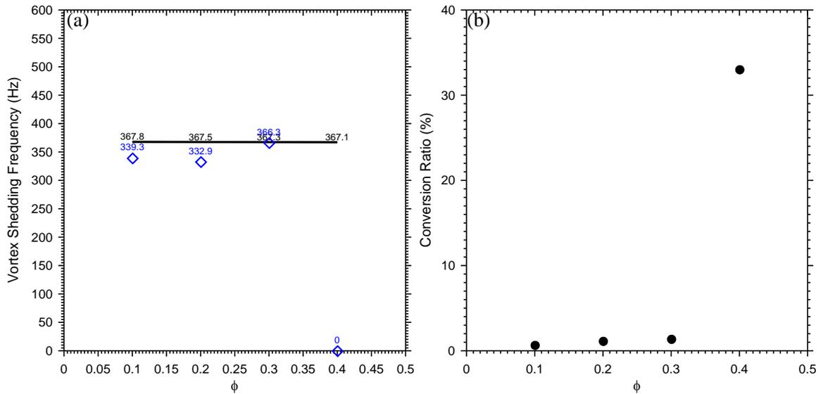
Figure 7 Vortex shedding frequency and conversion ratio for four cases
