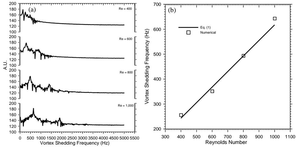
Figure 2 The vortex shedding frequencies with different Reynolds number for cold flow: (a) power spectrum; (b) comparison between theoretical and numerical predicted values
