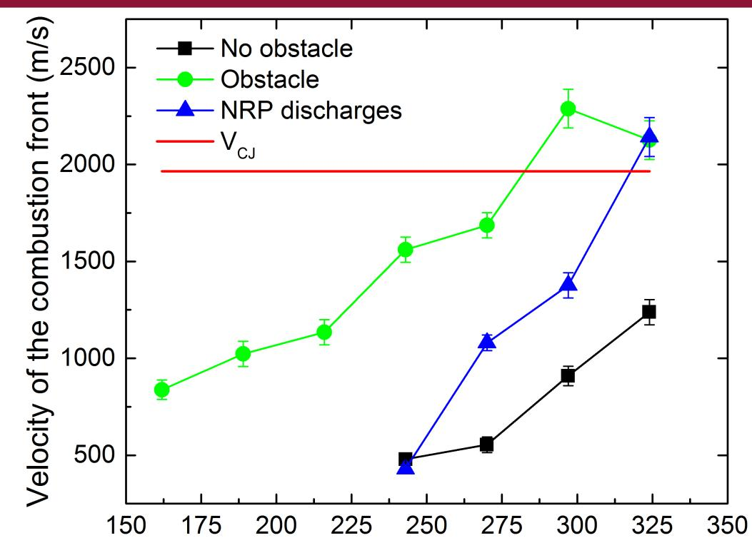
⇒ Effect of NRP glow discharges on the DDT of  $H_2$ -Air mixture: Proof-of-concept achieved for high-voltage NRP applied at 30 kHz, with a maximal voltage of 20 kV. In fresh mixtures, no discharge occurs, but after perturbation of the interelectrode volume by the propagation of pressure waves, there is generation of NRP spark discharges, able to enhanced the acceleration of the combustion front.
