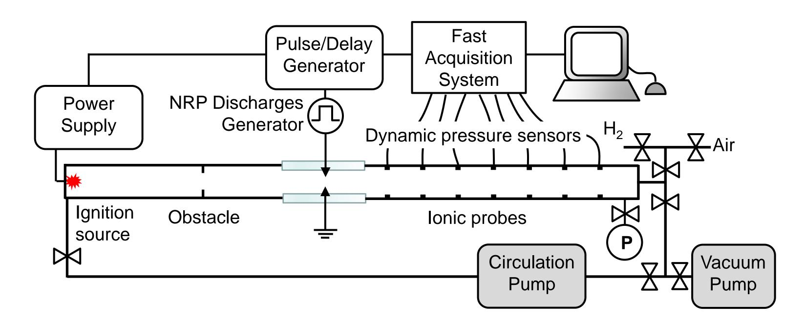
The experimental setup comprises a detonation tube equipped with a PMMA tube for optical access, an ignition system, and the system for generation of NRP discharges. All electrical systems, including acquisition, are synchronized. Below, a few characteristics:
