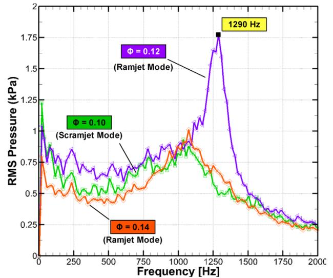
Figure 5. Close-up comparison of broadband pressure spectra for fueling conditions near transition regime.
