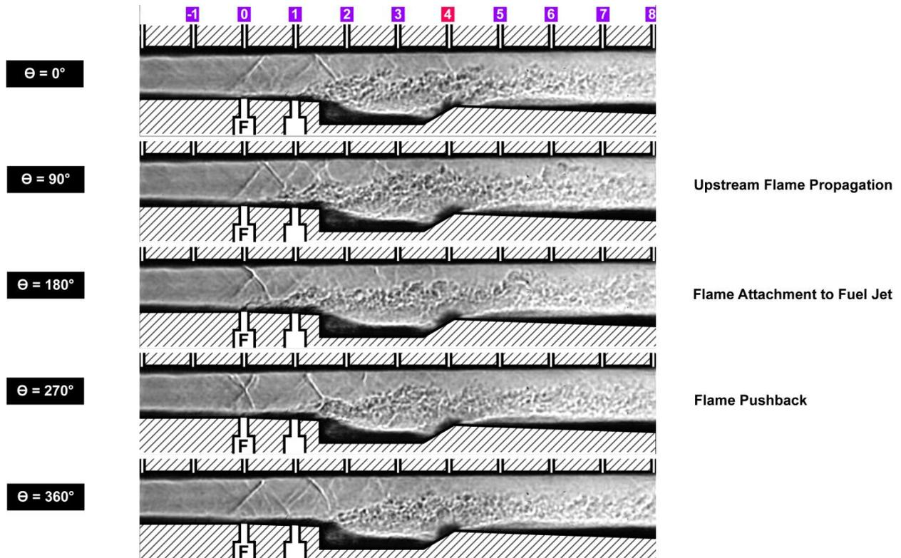
**Figure 6.** Selected images of a typical flame oscillation cycle for a  $\Phi = 0.10$ .
