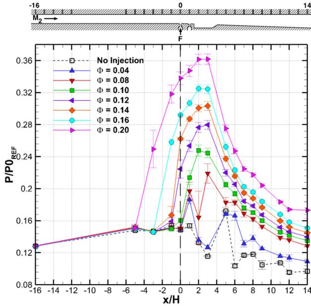
Figure 2. Time-averaged static pressure distributions through the flow path as a function of equivalence ratio.
