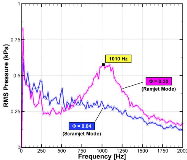
Figure 4. Close-up comparison of pressure spectra at lowest and highest fueling conditions tested.
