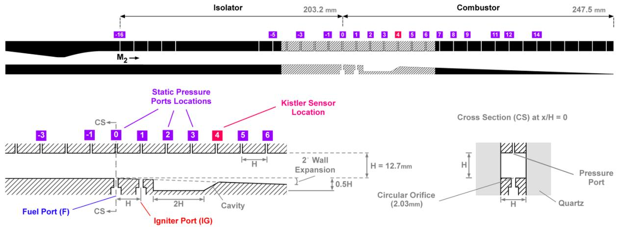
Figure 1. Cross-sectional schematic of flow path and detailed views of combustor test section.
