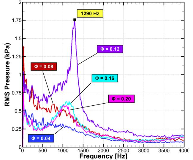
Figure 3. Pressure spectra obtained from FFT analysis of band passed-filtered dynamic pressure measurements.
