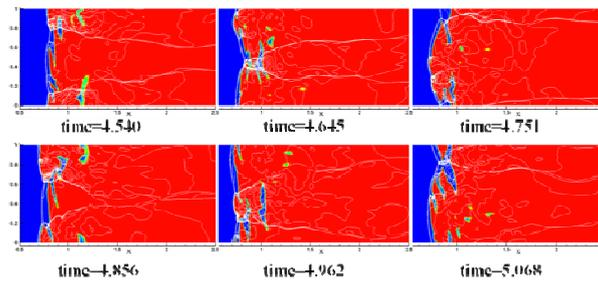
Figure 3. Pressure and reaction progress rate contours for  $k=4 \times 10^5$  at 2-D results.
