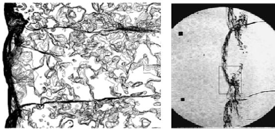
Figure 6. The pressure contour line is overlaid from  $y=0.7$  to  $y=0.75$  (left) and schlieren image by J. M. Austin in  $\text{C}_2\text{H}_4\text{-3O}_2\text{-8N}_2$ ,  $P_1=20\text{kPa}$  in the narrow channel (right).
