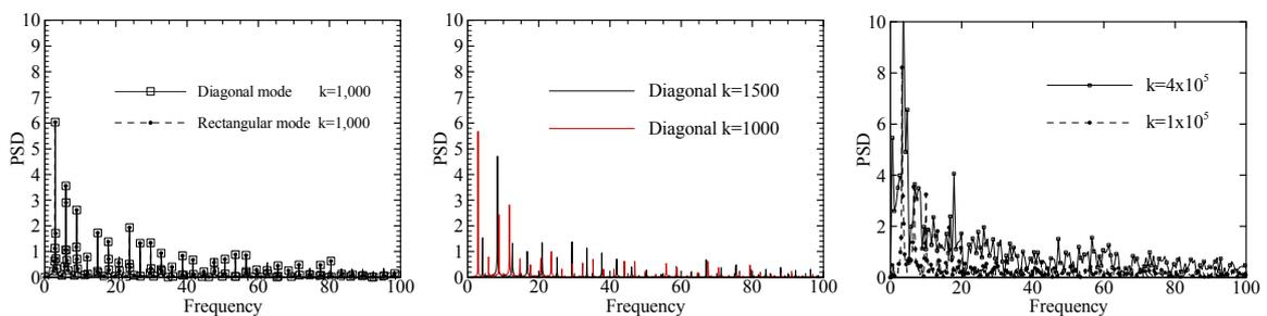
Figure 5. Amplitude of the oscillation mode as function of pre-exponential  $k$ . Weakly unstable results (left and middle) and highly unstable result (right)
