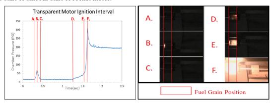
Figure 1. Hypergolic hybrid motor Ignition Interval Chamber Pressure
