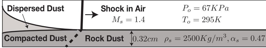
Figure 1: Schematic of shock wave propagating on top of and through a dust layer in a channel
