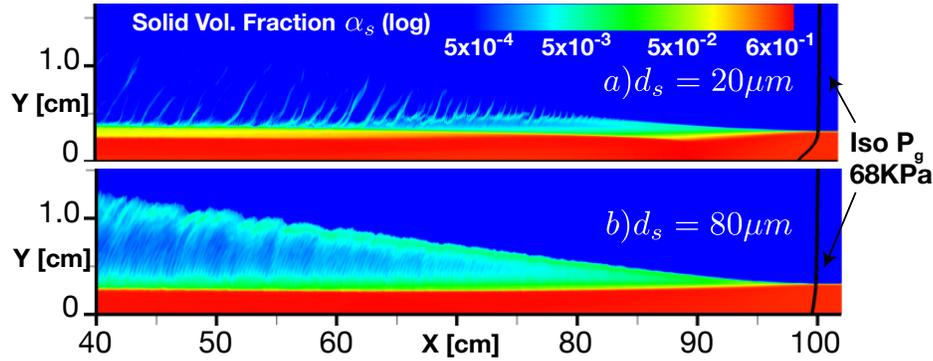
Figure 2: Variation of solid volume fraction behind a shock for 20  $\mu\text{m}$  and 80  $\mu\text{m}$  particles.
