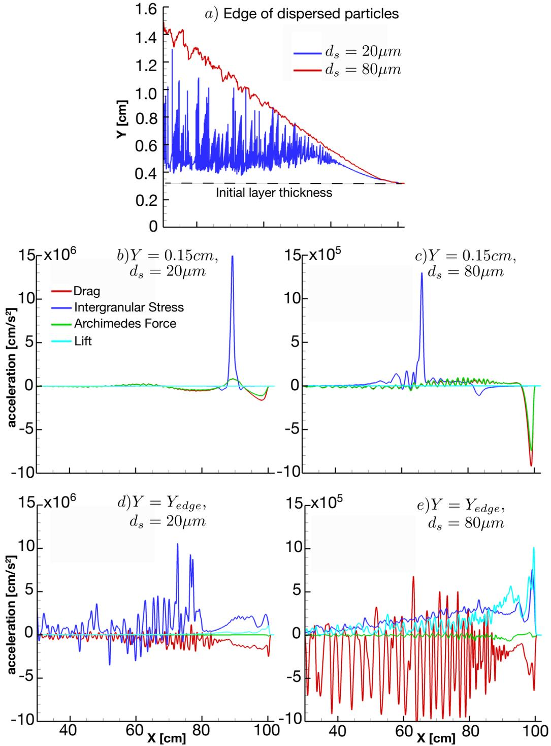
Figure 4: Height of the dispersed dust for 20  $\mu m$  and 80  $\mu m$  particles (a). Computation of forces listed in Table 1 inside the dust layer at  $Y = 0.15$  cm (b, c) and at the edge of the dispersed dust (d, e).
