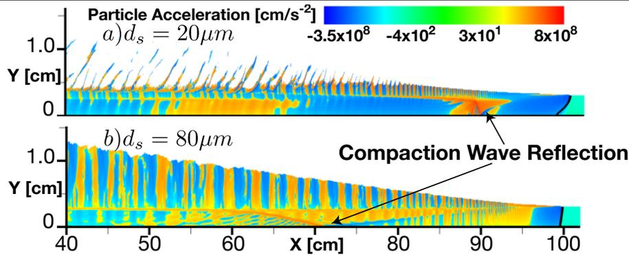
Figure 3: Vertical component of particle acceleration behind a shock, for 20  $\mu\text{m}$  and 80  $\mu\text{m}$  particles.
