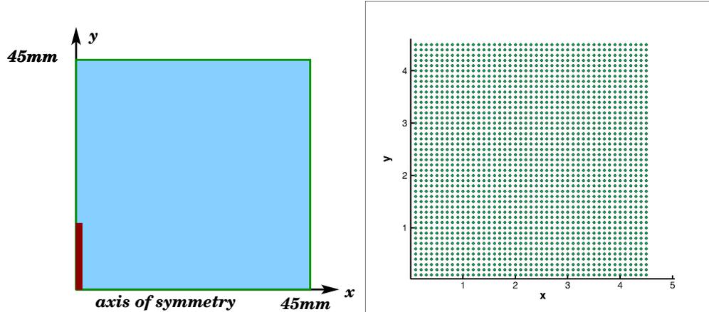
Figure 1: Left: the problem setup: the blue region is LX-17 at rest; the red disk is the detonation source (also LX-17) that has a radius of  $1.25\text{cm}$  and a thickness of  $0.1\text{cm}$ , with an initial velocity of  $0.75\text{ cm}/\mu\text{s}$  moving in the  $x$ -direction. The axis of symmetry is  $y = 0$ . Right: the locations of tracers where the shock arrival time is recorded. The spacing between neighbor tracers is  $h = 0.1\text{cm}$ .
