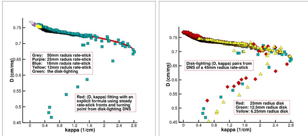
Figure 3: Left: the  $(D, \kappa)$  pairs extracted from the simulation with a disk-source with a radius  $1.25\text{cm}$ , and fitted with an analytic formula (the red curve) using steady rate-stick front geometries; right: similar  $(D, \kappa)$  pairs obtained with three different source radii. Their turning points share nearly the same location.
