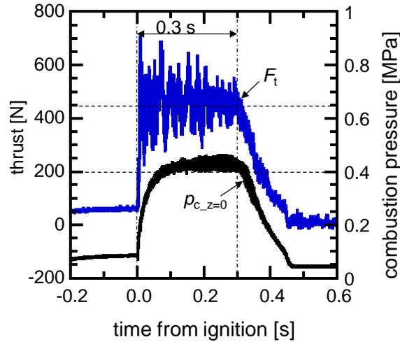
Fig. 3 Thrust and combustion pressure of sh#2\_vac.
