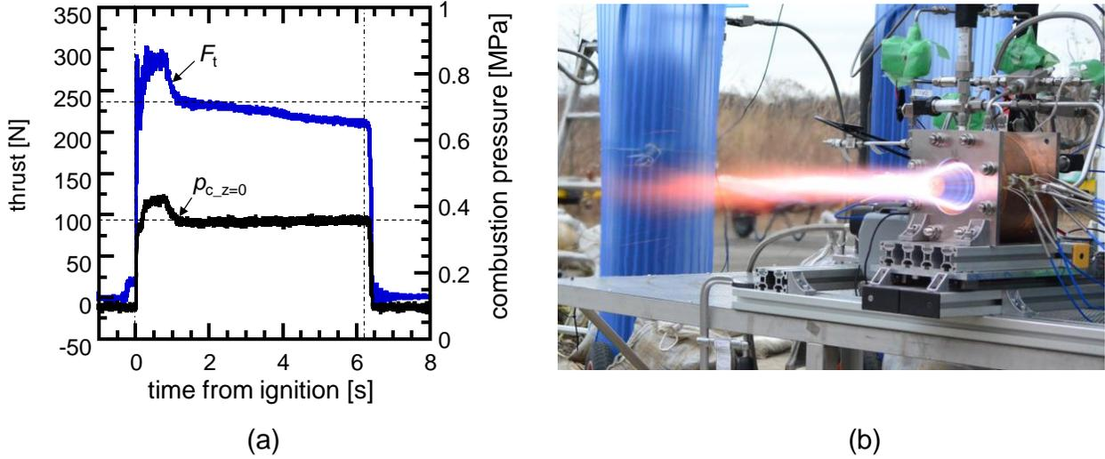
Fig. 5 Experimental results (a) thrust and combustion pressure (b) a picture during combustion test
