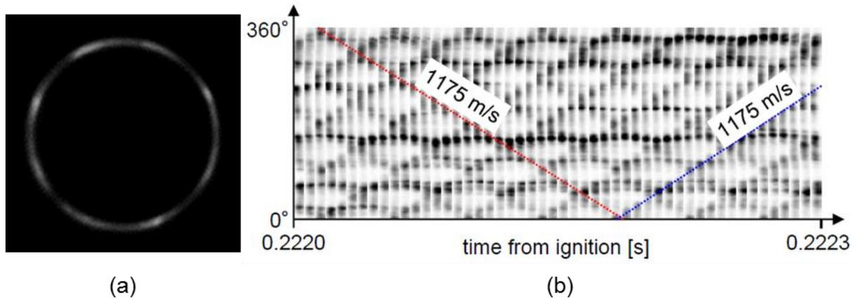
Fig. 4 Visualized images (a) self-emission of detonation waves
