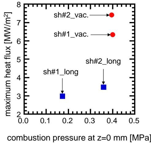
Fig. 6 Influence of the combustion pressure on heat flux
