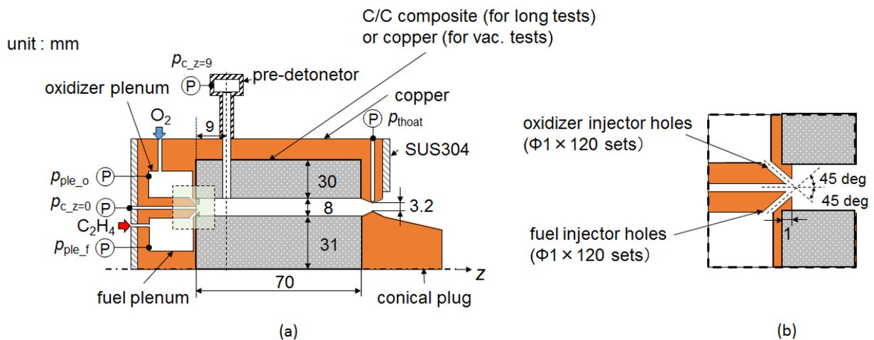
Fig. 1 (a) Schematic of the RDE, (b) Enlarged view around the injector
