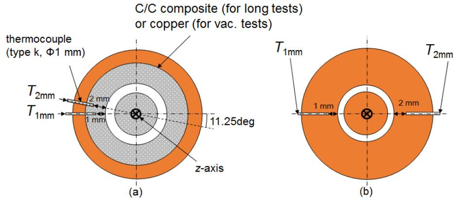
Fig. 2 Placement of the thermocouples, (a) cross sectional view at  $z=2, 9, 18, 35, 65$  mm, (b) at the throat
