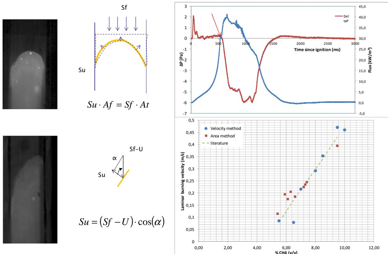
Figure 2 : laminar burning velocity methods
