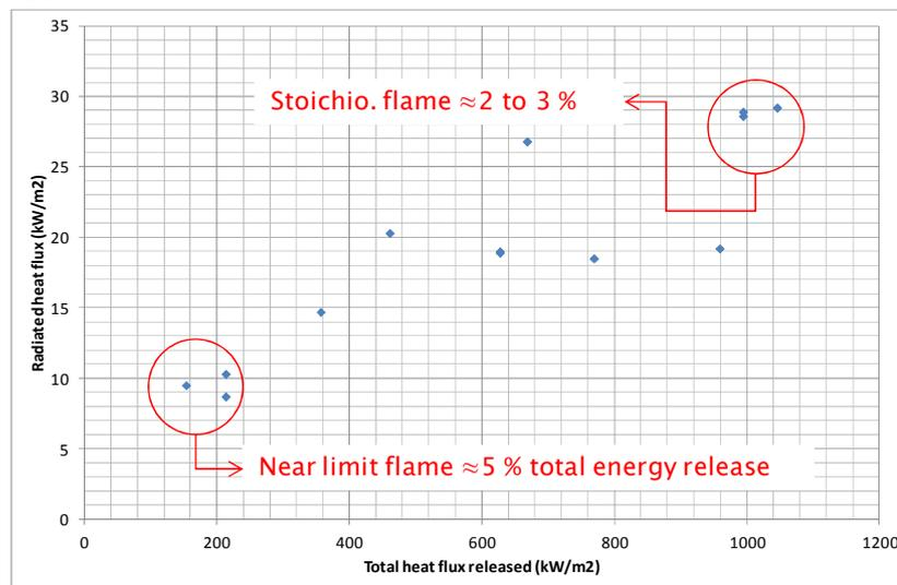
Figure 3. radiated heat flux as function the total heat flux released (methane air flame)<sup>1</sup>
