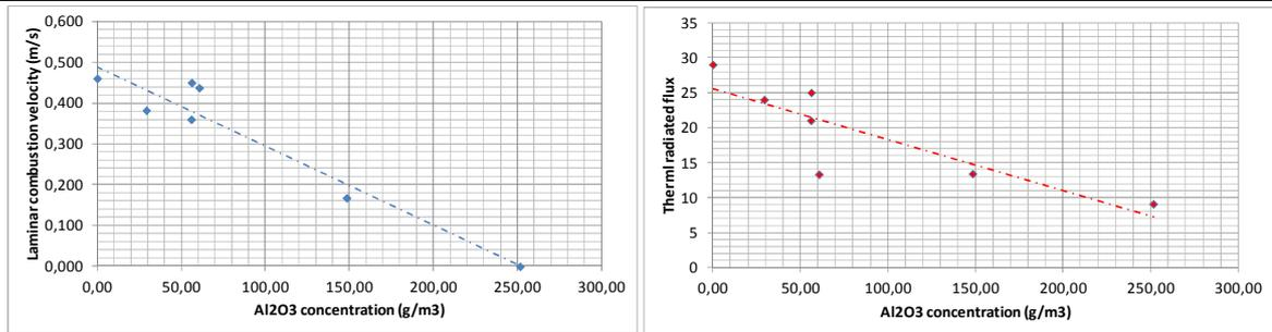
Figure 4. methane air flame (stoichiometry) seed with alumina particles
