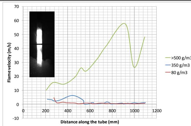
Figure 6 : self acceleration of flames propagating in a aluminium dust-air cloud
