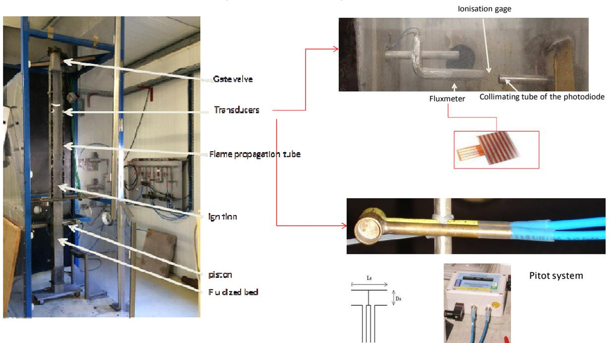
Figure 1. Experimental setup
