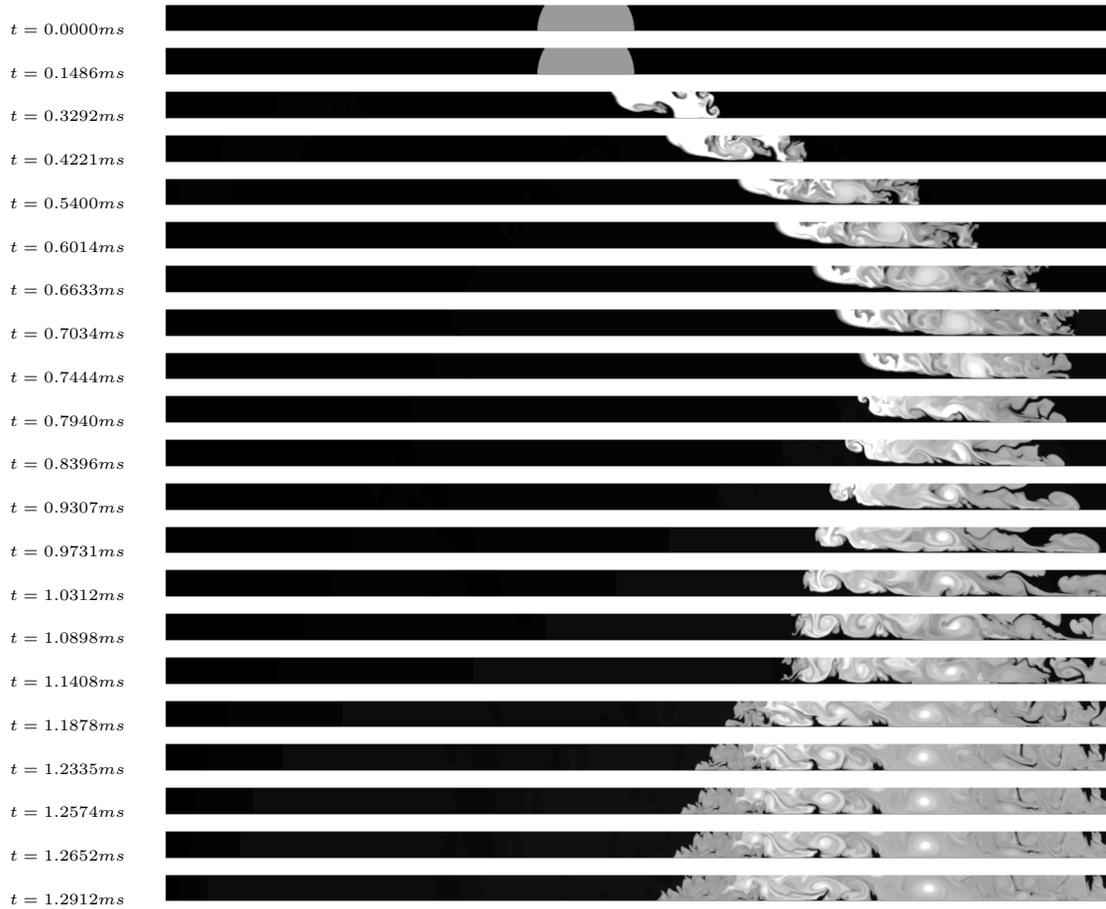
Figure 2: Time-sequence of temperature contours for an incident shock at  $Ma = 1.5$ . Colour legend: 65 levels,  $min = 400K$ ,  $max = 3600K$ .
