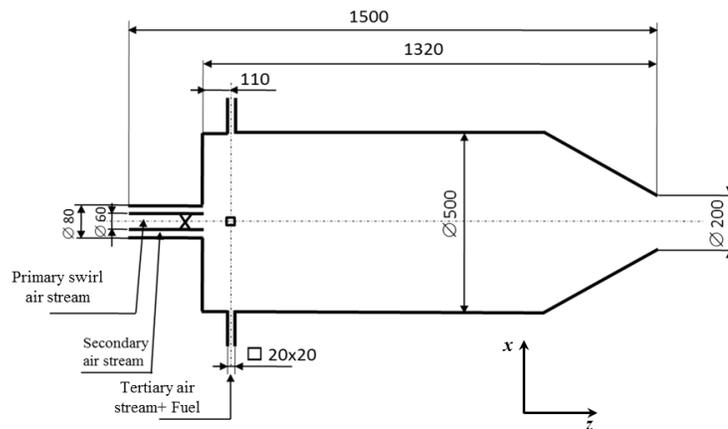
Figure1. Schematic view of computational domain (mm)
