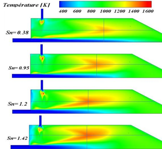
Figure 3. Gas temperature for different swirl numbers ( $S_n$ ) (plan x-z)
