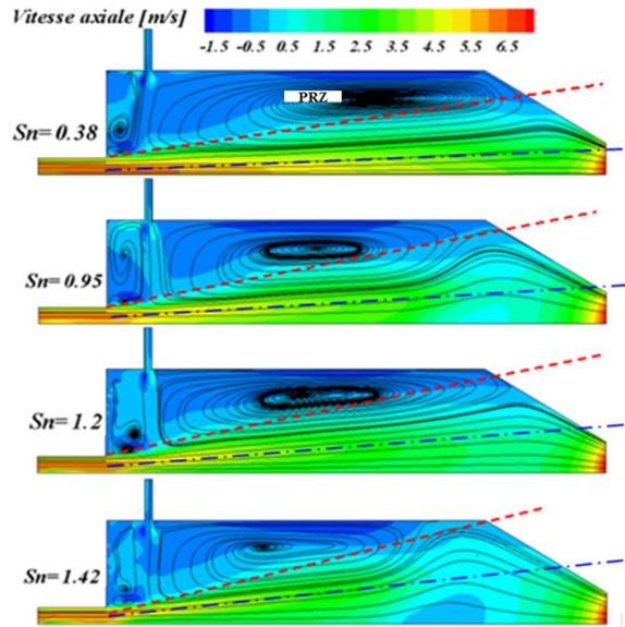
Figure 2. Streamlines and average axial velocity for different swirl numbers ( $S_n$ ) (plan x-z)
