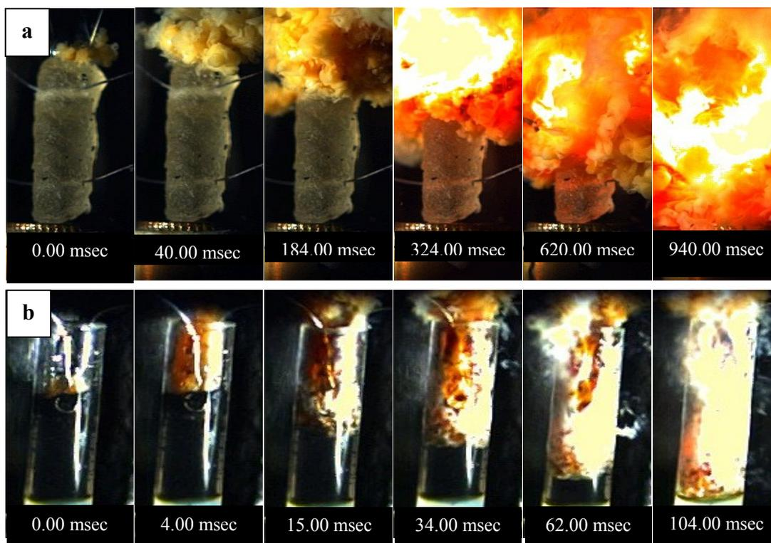
Figure 2. Captured images of regression process during combustion of HAN based propellant with various additives. (a) HAN-based propellant containing 10 wt % Carboxymethyl cellulose gel at 50 atm.,  $r_b = 32.05 \text{ mm/s}^{-1}$ . (b) HAN-based propellant containing 1 wt % Activated carbon (CRH-K<sub>2</sub>CO<sub>3</sub>) at 50 atm.,  $r_b = 143.6 \text{ mm/s}^{-1}$ .
