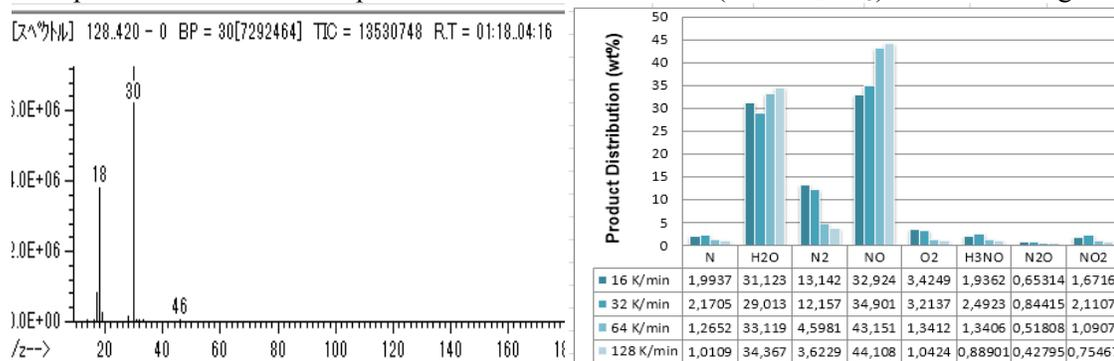
Figure 4. MS analysis of HAN decomposition with activated carbon CRH-475 K<sub>2</sub>CO<sub>3</sub> and the product distribution at 64 K/min heating rate.
