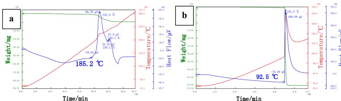
Figure 3. DTA-TG analysis results of HAN decomposition at 20 K/min heating rate
