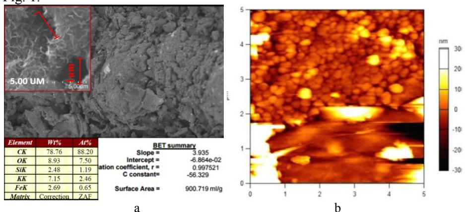
Figure 1. Scanning electron microscope image and BET analysis (a) and atomic-force microscopy (b) of morphology structure of CRH- $\text{K}_2\text{CO}_3$ -475 activated carbon
