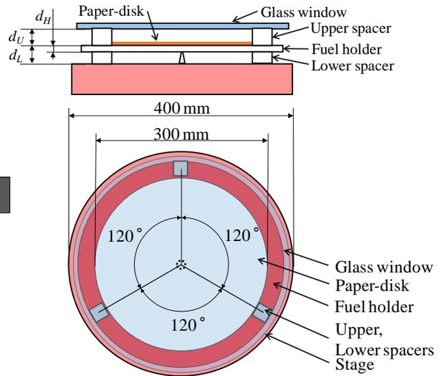
Fig. 2. Diagram of test section
