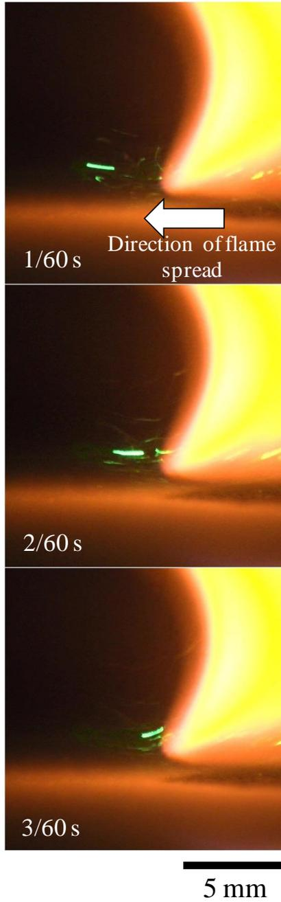
Fig. 7. Visualization of flow by using PIV technique in the upper gap
