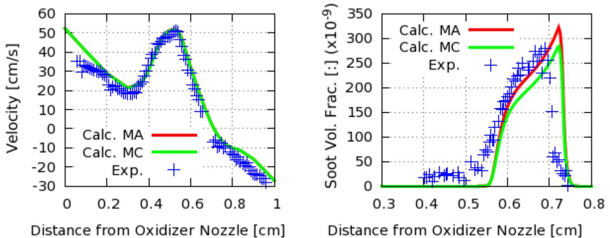
Figure 2. (Left) Experimental velocities for flame 3 in Ref. [4] compared to results obtained with mixture-average (MA) and multi-component transport model (MC). (Right) Soot volume fraction comparison for the same cases.
