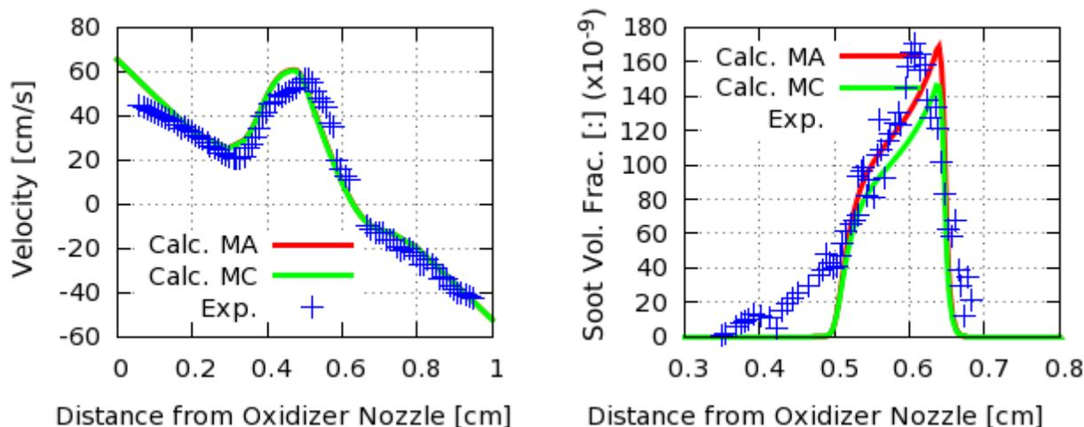
Figure 1. (Left) Experimental velocities for flame 1 of Ref. [4] compared to calculated results obtained with mixture-average (MA) and multi-component transport model (MC). (Right) Soot volume fraction comparison for the same cases.
