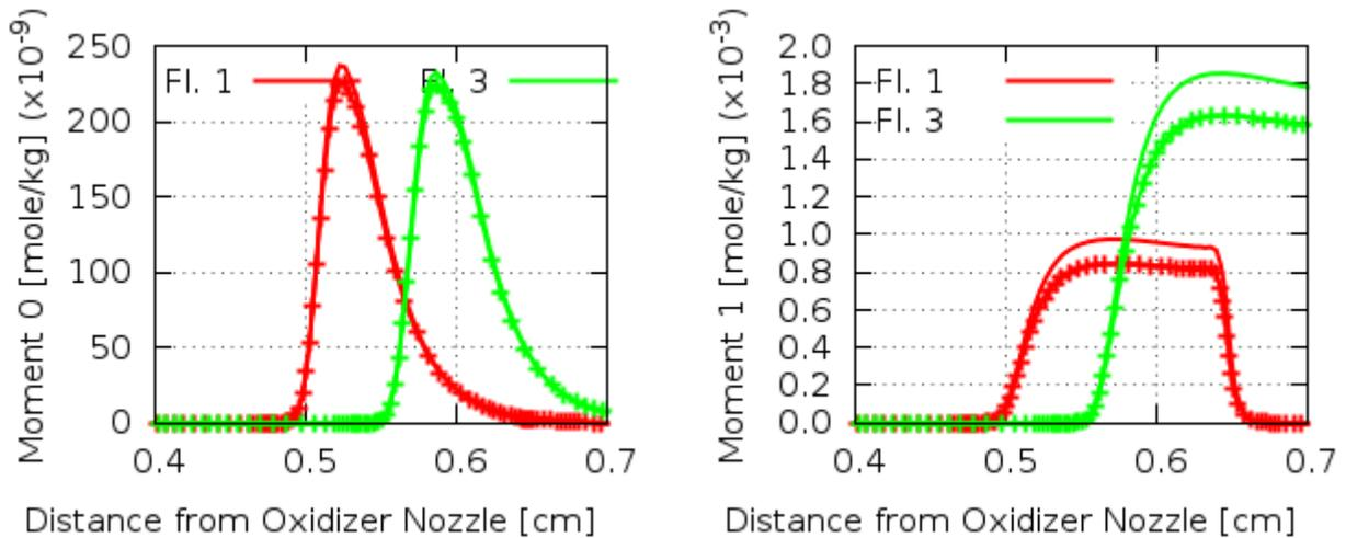
Figure 3. Calculated soot moment 0 (Left) and soot moment 1 (Right) of flames 1 and 3. Dashed lines indicate multi-component calculation while solid lines show mixture-averaged calculation.
