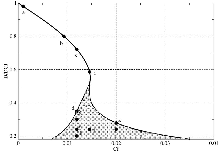
Figure 1:  $D - c_f$  dependence for detonation with  $Q = 50$ ,  $E = 25$ ,  $\gamma = 1.2$ ,  $c_h = 0.4c_f$ . Points  $c - h$  correspond to  $c_f = 0.012$ .
