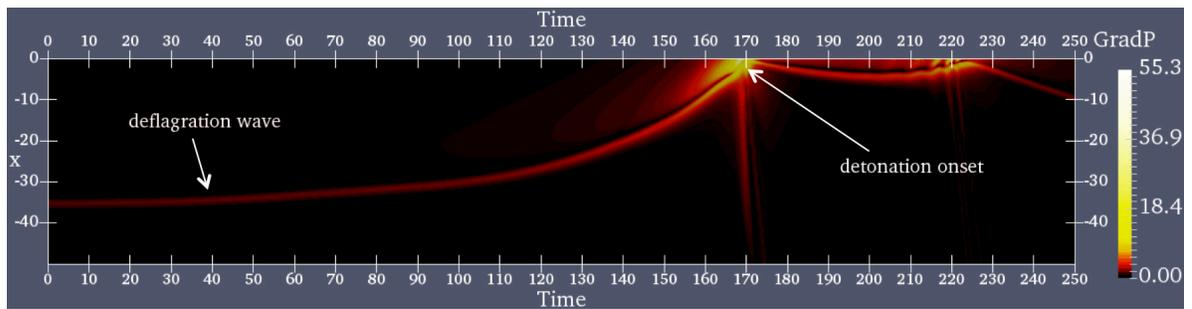
Figure 4: Space-time depiction of the transition process from the set-valued to the high-velocity regime. The parameters are:  $D/D_{CJ} = 0.3$  for the steady state,  $E = 25$ ,  $Q = 50$ ,  $\gamma = 1.2$ ,  $c_f = 0.012$ ,  $c_h = 0.4c_f$ . The computational domain of length  $L = 1000$  with resolution of  $N_{1/2} = 100$  points per half-reaction length was used.
