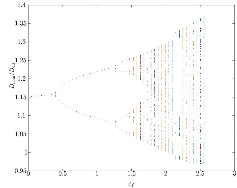
Figure 2: Bifurcation diagram for detonation with losses showing the maximum of  $D$  in the limit cycle as the friction coefficient is varied. The other parameters are  $Q = 50$ ,  $E = 27$ , and  $\gamma = 1.2$ .  $D_{CJ}$  is the ideal velocity at these parameters.
