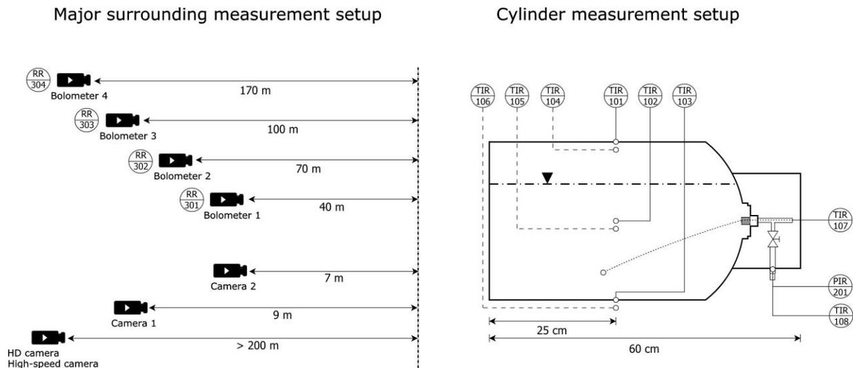
Fig. 1: Schematic diagram of the experimental and measurement set-up and the instrumentation for the bonfire tests of the propane cylinders
