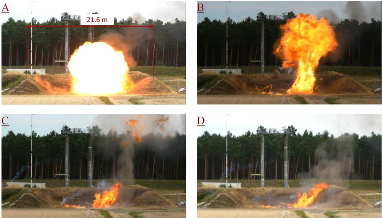
Fig. 2: Sequence of failure of a propane cylinder and the subsequent explosion of the gas cloud; approximately 0.5 s (A) / 1.5 s (B) / 2.5 s (C) / 3.5 s (D) after the rupture of the vessel (cf. Fig. 3a), wood fire, test pc-02
