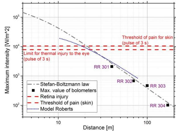
Fig. 3b: Maximum intensity of the infrared radiation, comparison between the maximum heat flux calculated using the Stefan-Boltzmann law applied to the video data of the fireball, the measurements using the bolometers (RR 301 to 304, cf. Fig. 1) and BLEVE model according to Roberts (cf. [10]), wood fire, test pc-02
