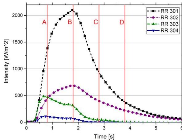
Fig. 3a: Intensity of the infrared radiation recorded by the bolometers (in distances of 40 m and 70 m to the vessel using slow bolometers RR 301 and RR 302, in distances of 100 m and 170 m using fast bolometers RR 303 and RR 304), wood fire, test pc-02, cf. Fig. 2 regarding points A to D
