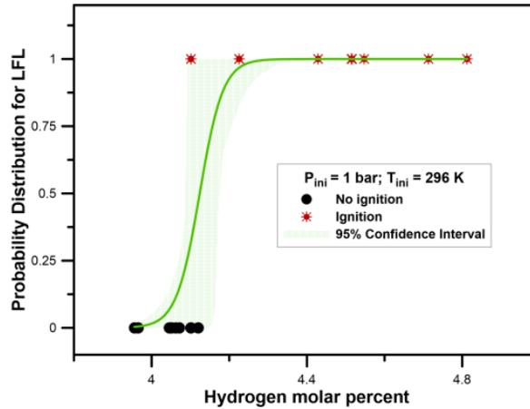
Figure 1. Probability distribution for tests of H<sub>2</sub>/O<sub>2</sub> mixtures initially at 1 bar and 296 K
