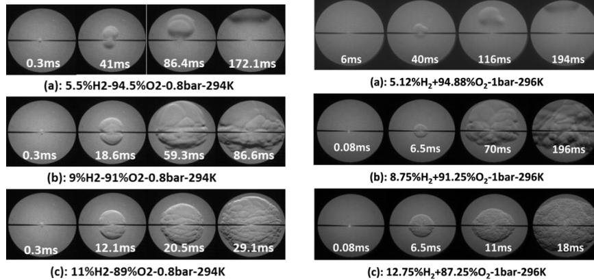
Figure 2. Type of lean flame propagation of  $H_2/O_2$  mixture at 1 bar and 296 K.
