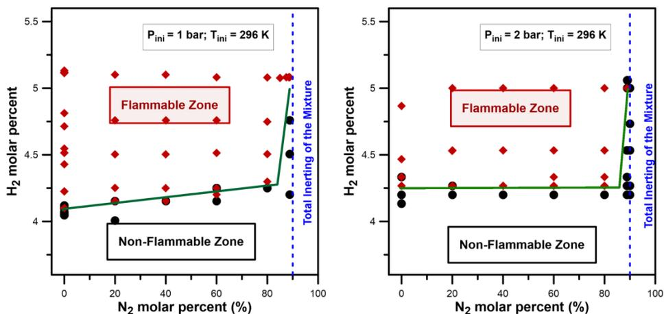
Figure 5. Evolution of the flammability limit with the N<sub>2</sub> dilution. (Left): 1 bar and 296 K; (Right): 2 bar at 296 K.
