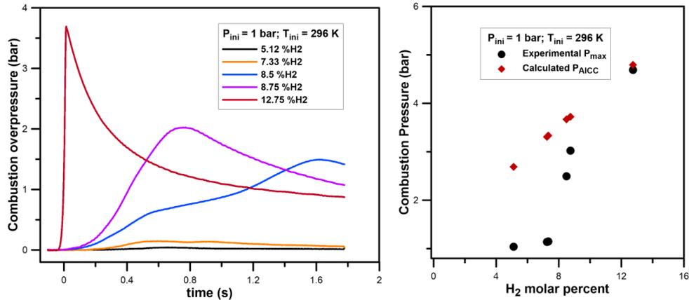
Figure 4. Evolution of the experimental combustion overpressure versus time (left) and theoretical ( $P_{AICC}$ ) and experimental maximum pressure ( $P_{max}$ ) versus the hydrogen molar percent (right) at 1 bar and 296K.
