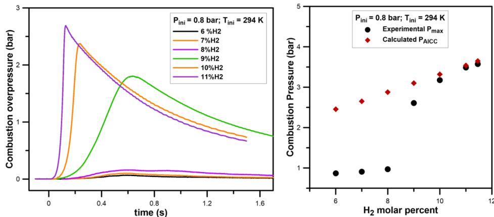
Figure 3. Evolution of the experimental combustion overpressure versus time (left) and theoretical ( $P_{AICC}$ ) and experimental maximum pressure ( $P_{max}$ ) versus the hydrogen molar percent (right) at 0.8 bar and 294K.
