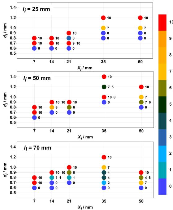
Figure 3: Re-ignition frequency maps for  $l_i = 25$  mm,  $l_i = 50$  mm and  $l_i = 70$  mm. Colorbar: Number of re-ignitions within 10 experiments.
