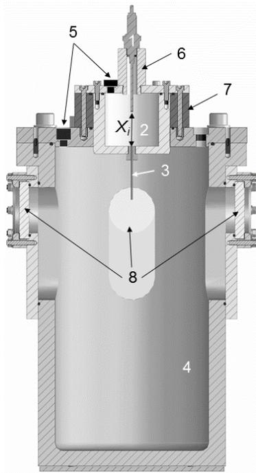
Figure 1: **Test chamber.** The pre-chamber (diameter 70 mm, volume 0.267 l) is connected by a nozzle with the main chamber measuring an inner diameter of 200 mm (height, 367 mm, volume 11.5 l).
