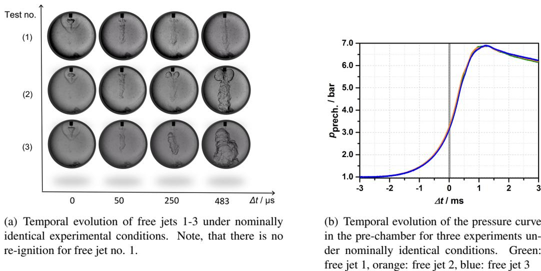
Figure 4: (a) Three tests with identical experimental configurations ( $l_i = 70$  mm,  $d_i = 1.0$  mm and  $X_i = 35$  mm) lead to re-ignition in two cases (jets 2 and 3) and to no re-ignition in another (jet 1). (b) However, all three pressure curves in pre-chamber have an identical shape.
