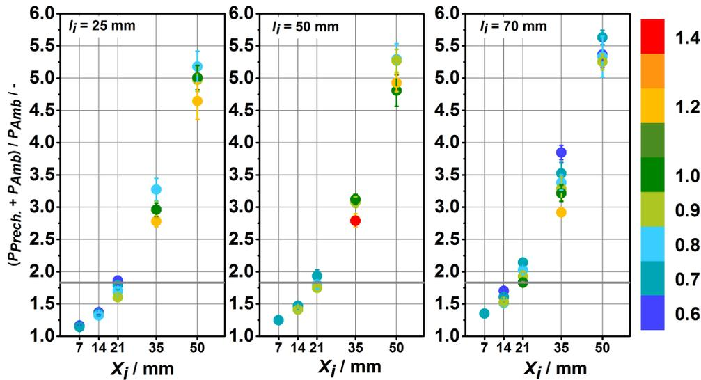
Figure 5: Mean pressure ratio of pressures in the pre-chamber and the main chamber as a function of spark plug distance  $X_i$  and nozzle diameter  $d_i$  for nozzle lengths  $l_i = 25$  mm, 50 mm and 70 mm. ( $X_i = 35$  mm,  $l_i = 25$  mm and  $d_i = 0.9$  mm and 1.0 mm, based on 9 tests;  $X_i = 35$  mm,  $l_i = 70$  mm and  $d_i = 0.6$  mm, based on 8 tests).
