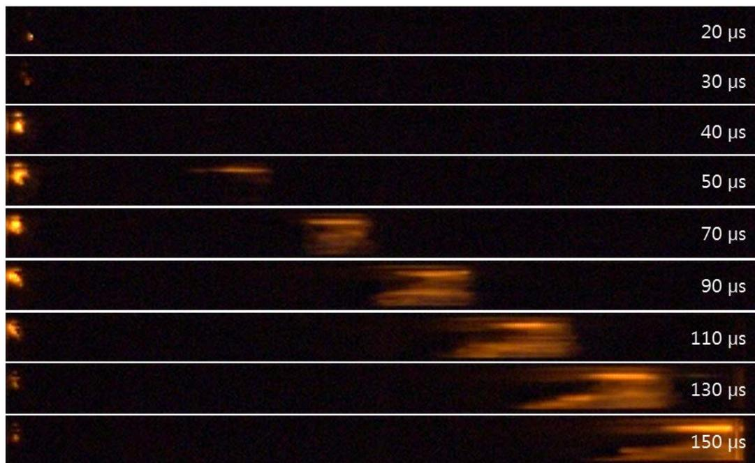
Fig. 3 Direct image at burst pressure of 11 MPa (open area ratio of 1.0)
