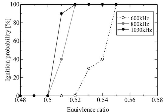
Figure 4. Ignition probability for methane/air mixtures at 100kPa.
