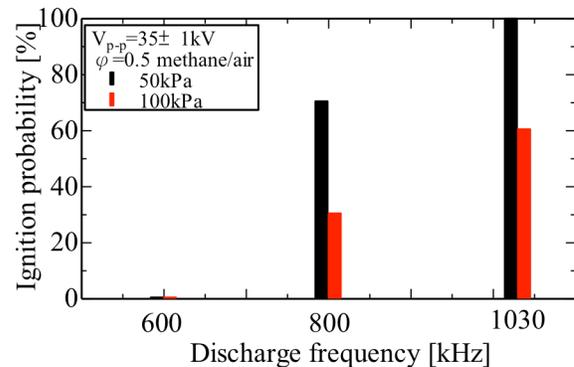
Figure 6. Ignition probability for methane/air mixtures with the equivalence ratio of 0.5 under the same discharge counts.
