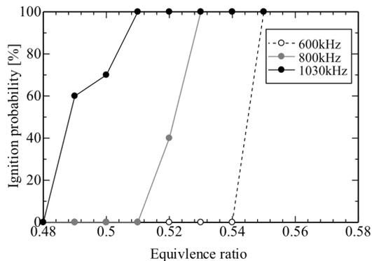
Figure 5. Ignition probability for methane/air mixtures at 50kPa.
