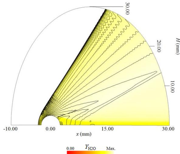
Figure 1. Overlaid contours of ODW structure in a uniform flow
