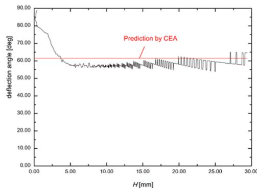
Figure 2. Profile of ODW front angle in the uniformly premixed condition
