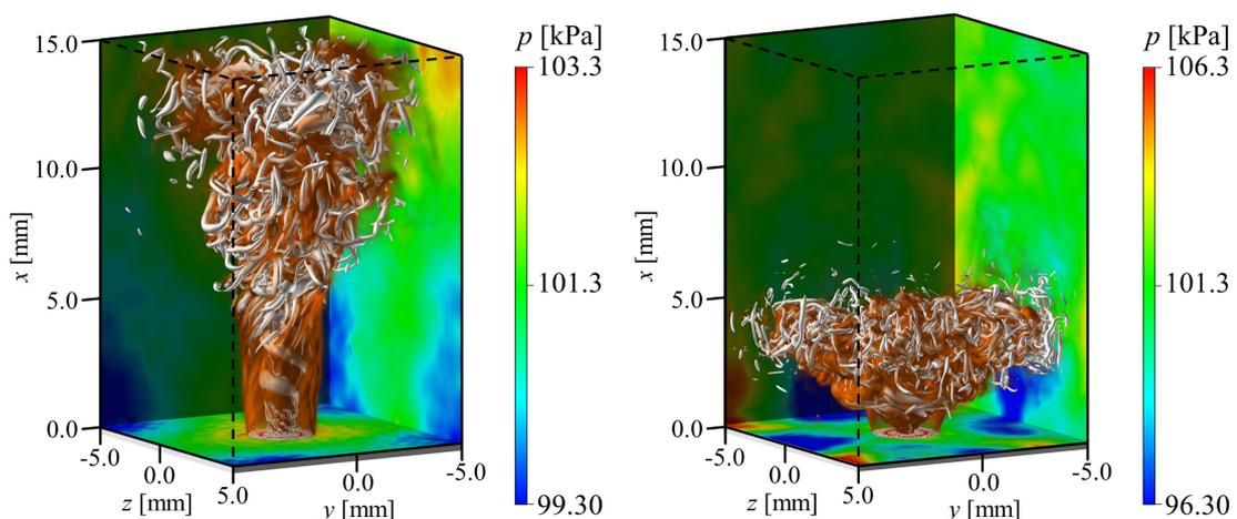
Figure 1. Instantaneous iso-surfaces of the second invariant of a velocity gradient tensor (iso-surfaces at 1% of a maximum value are visualized), volume rendered  $\omega_T$ , and distribution of  $p$  on the walls (left:  $S = 0.6$ , right:  $S = 1.2$ ).
