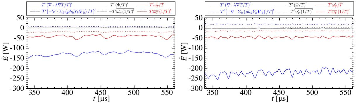
Figure 4. Components of source term  $D_Q$  related to heat transfer fluctuation (left:  $S=0.6$ , right:  $S=1.2$ ).
