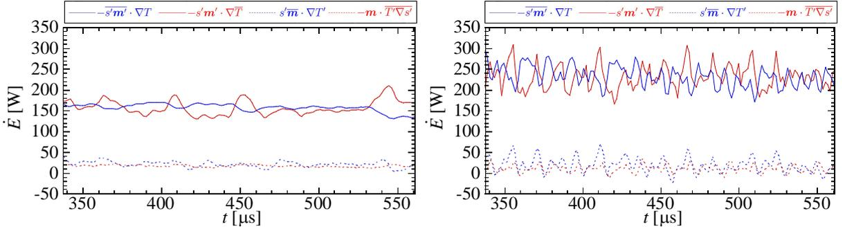
Figure 3. Components of source term  $D_s$  related to entropy fluctuation (left:  $S=0.6$ , right:  $S=1.2$ ).
