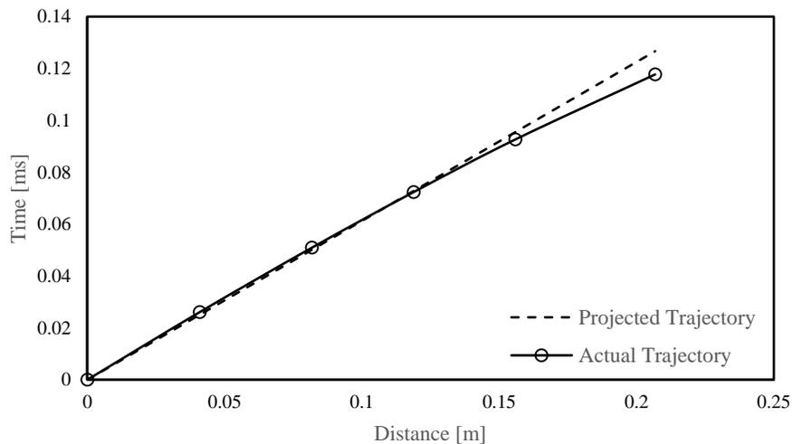
Figure 2a: x-t Diagram for  $C_2H_2+2.5O_2+70\%$  Argon of  $10^\circ$  Convergence at 6kPa
