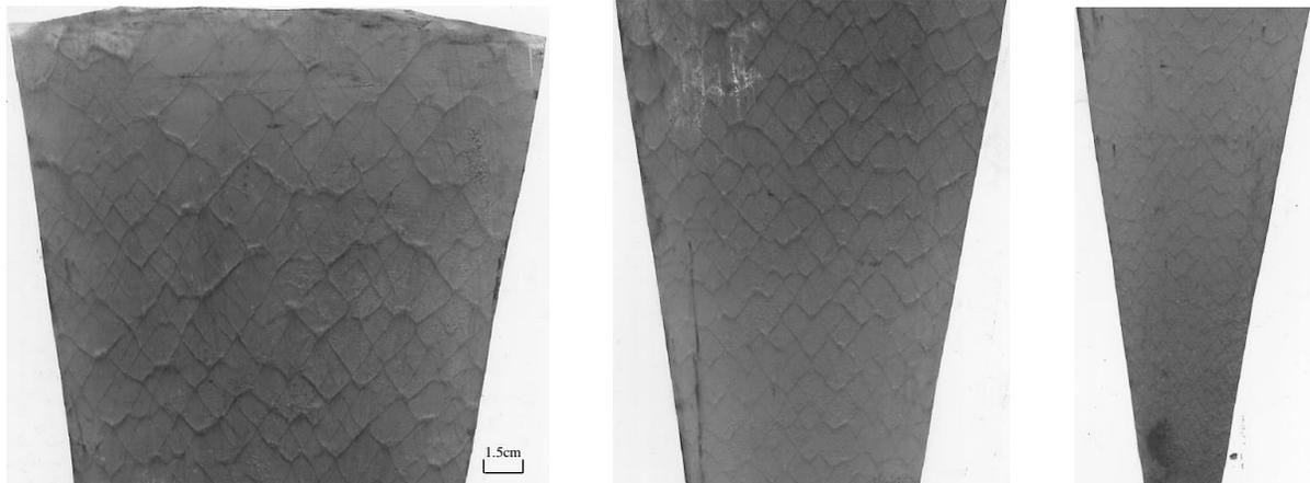
Figures 3a, 3b and 3c: Smoked Foils for  $C_2H_2+2.5O_2+70\%$  Argon at  $6^\circ$  Convergence and 6kPa
