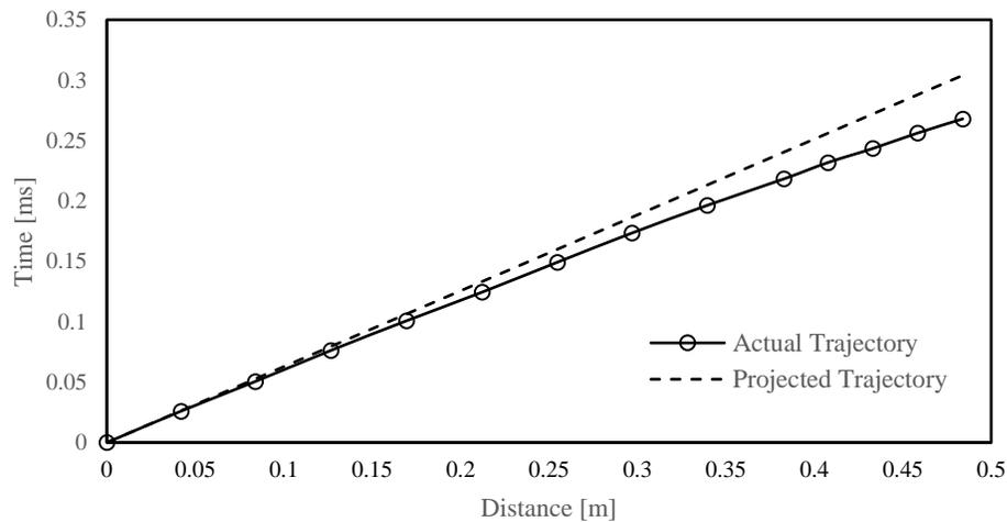
Figure 2b: x-t Diagram for  $C_2H_2+2.5O_2+70\%$  Argon of  $6^\circ$  Convergence at 6kPa
