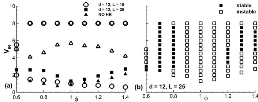
Figure 2. (a) Flammability limits and (b) flame stability regime diagram, stable and unstable flame shown by filled and unfilled symbols respectively.
