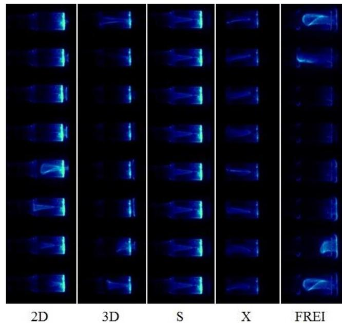
Figure 3. Instantaneous flame photographs for different type of flames observed. Each column shows six instantaneous images over a period of cycle. *2D* is for only pulsating flame, *3D* for flame having simultaneous pulsating and rotational motion, *S* for stable anchored flame, *X* (flame seen by naked eye as letter 'x') for rotating flamelet and *FREI* for flame repetitive extinction and ignition.
