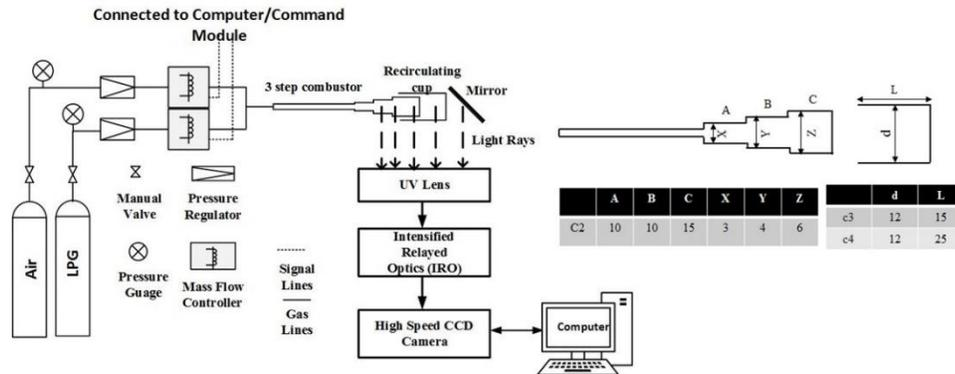
Figure 1. Experimental set up and combustor dimensions (mm).
