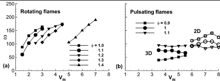
Figure 4. Behavior of frequency with mixture inlet velocity for (a) rotating flames and (b) pulsating flames
