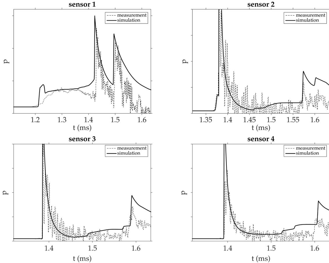
Figure 1: Pressure evolution of the adapted numerical simulation at the measurement positions, see Fig. 2(a). A very good agreement to the experimental data is found. The pressure signals match in terms of phase and amplitude.
