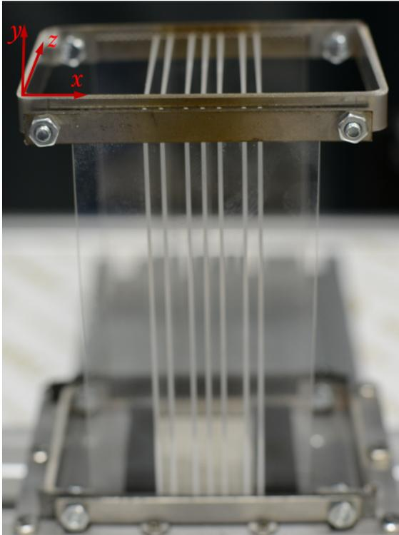
Fig.1. Photograph of the multi-channel burner.
