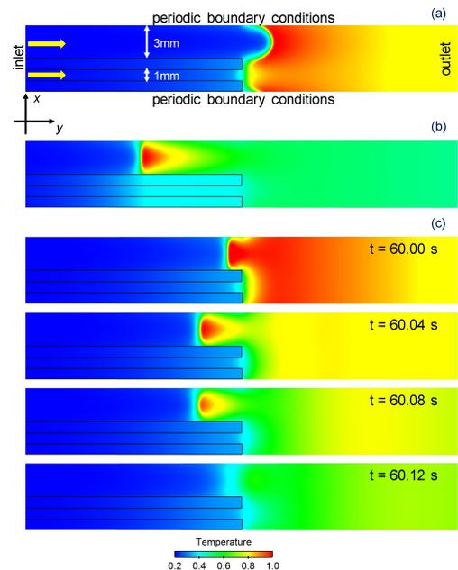
Fig.2. Temperature distributions for different combustion modes in configuration III calculated for  $Q = 285 \text{ cm}^3/\text{s}$  (a),  $Q = 125 \text{ cm}^3/\text{s}$  (b) and  $Q = 95 \text{ cm}^3/\text{s}$  (c).
