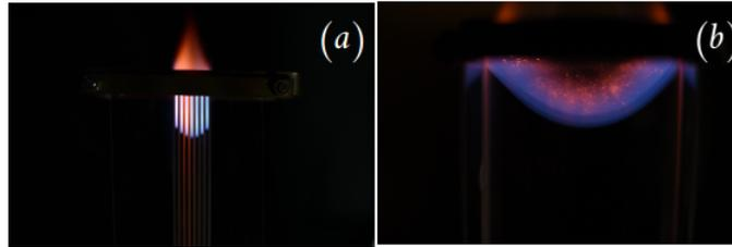
Fig.4. Front and side views of the flames stabilized inside the channels at  $\phi=1$ ,  $Q=202.5 \text{ cm}^3/\text{s}$ .
