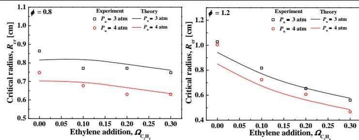
Figure 5. Measured and theoretical critical radius with various mixing ratio and elevated pressure
