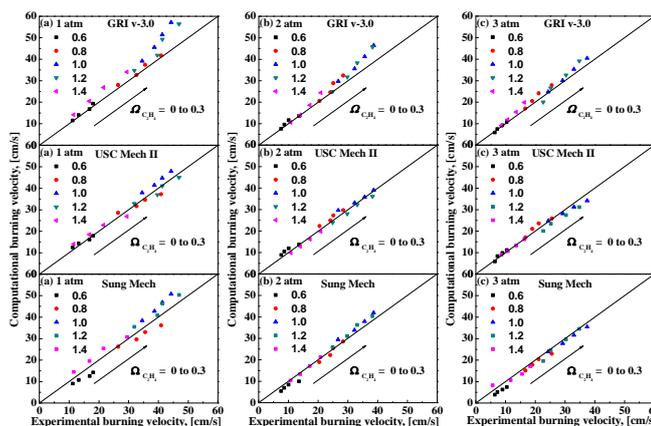
Figure 3. Comparison of Laminar burning velocities between experiment and calculation with variation of detailed mechanisms at 1 (a), 2 (b), and 3 (c) atm.
