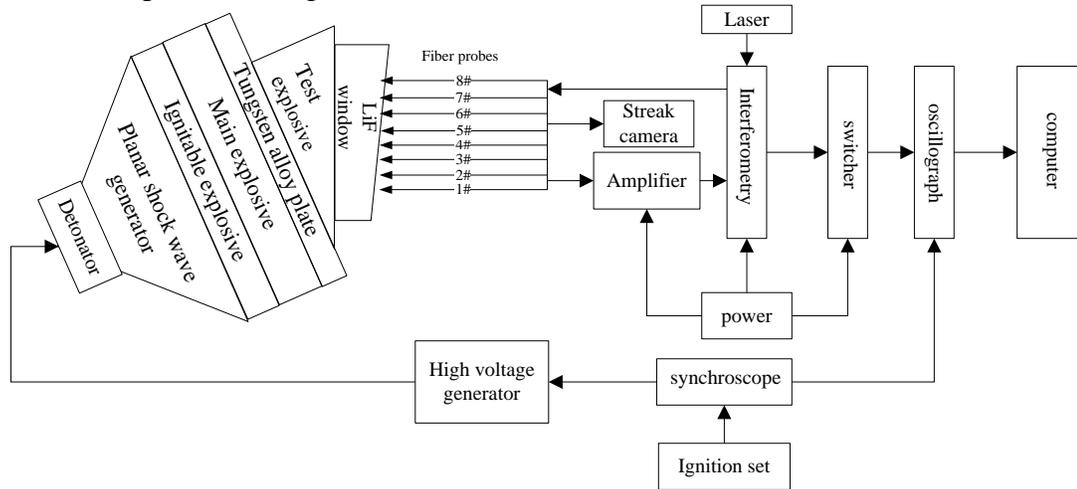
Figure1. The sketch of Experimental setup and measurement system
