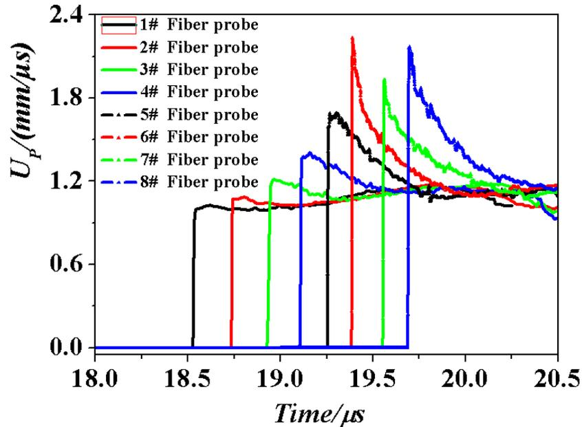
Figure3. Particle velocity profiles at the TATB-based Explosive /LiF interface obtained by Photon Doppler Velocimetry
