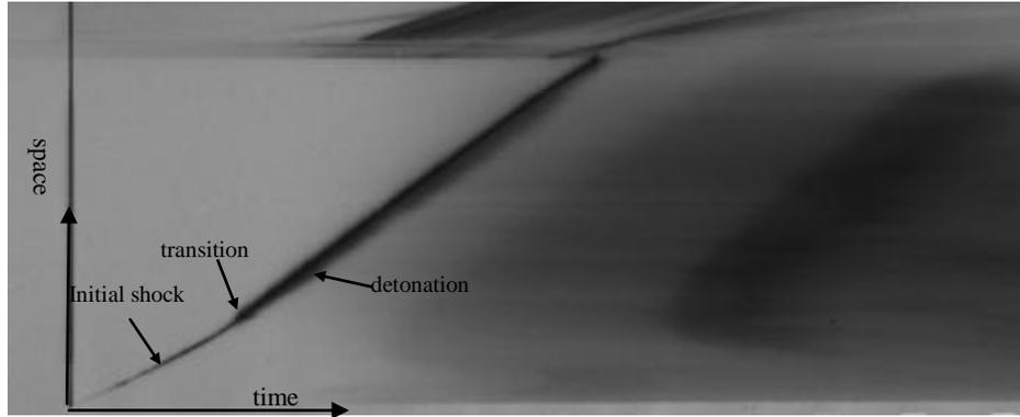
Figure2. High speed rotating mirror streak camera record and its interpretation
