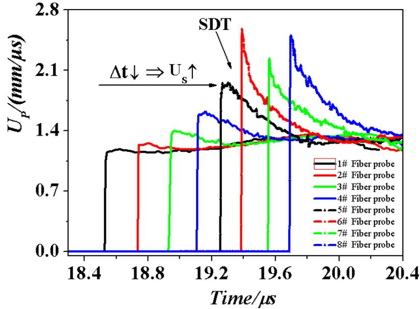
Figure4. Particle velocity profiles of JBO9021
