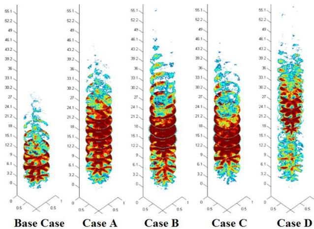
Figure 1. Flame natural luminosity profiles as a function of CAD for all cases considered
