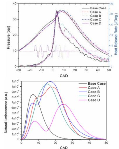
Figure 2. In-cylinder pressure and accumulated heat release rate profiles (top) and integrated natural luminescence signal for all cases considered (bottom)
