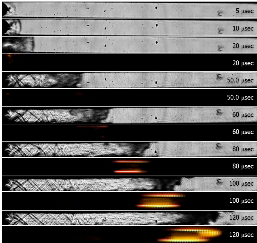
Fig. 4 Visualization image at burst pressure of 90 bar (open area ratio of 1.0)
