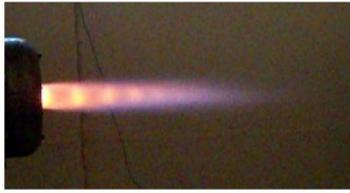
Fig.22 Flame jet propagating from aft end of 2-stage rig (Model 1)
