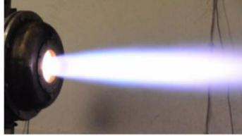
Fig.23 Image of the flame structure of second model of combustion (Model 2)
