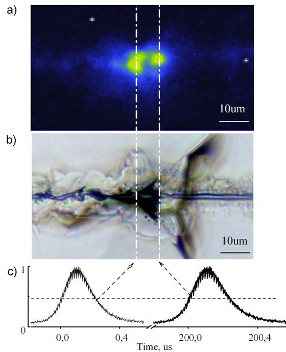
Figure 2. The micrographs of the region with the start and stop points: a) the plasma glow during damaging F3
