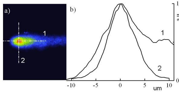
Figure 5. The high-speed micrograph of the laser plasma in the core of F3: a) the 2ns exposure time micrograph of the plasma propagated from right to left with speed of 2.8um/ns, b) the glow intensity curves.
