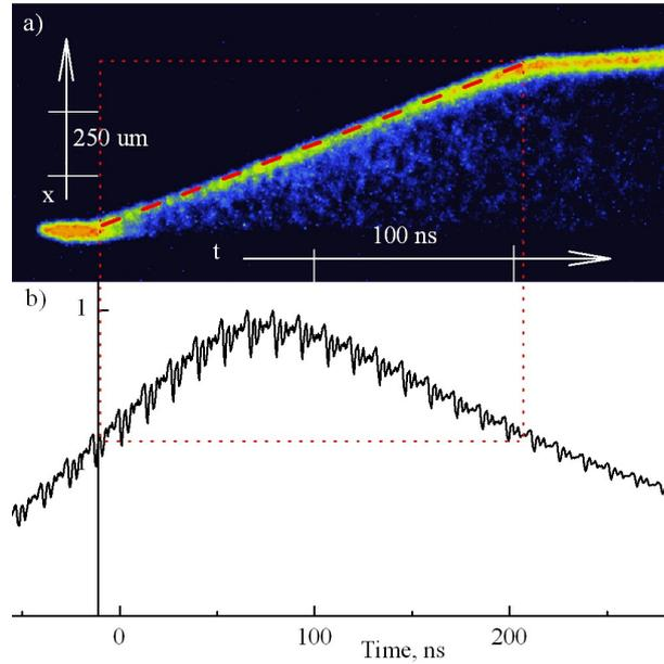
Figure 3. The plasma propagation in the F2 fiber core under laser pulse: a) the streak camera image, b) the oscilloscope picture of the laser intensity (in arbitrary units). The red dashed line has been laid throughout the maximums of plasma glow.
