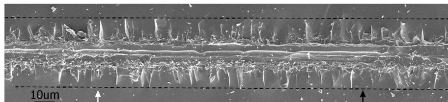
Figure 7. Radial cracks on the detonation channel in F2. Middle of detonation track is marked with a black arrow. Dotted lines are drawn through the ends of the RC. A change in the length of the RC pointed white arrow. Destruction moves from right to left.
