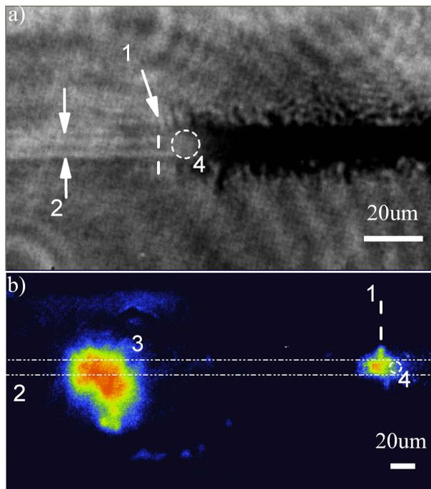
Figure 6. The high-speed micrograph of LSD (the 2ns exposure time): a) shadow picture of F2, b) in-crossed-polarizers picture of F3. 1 - the cross-section plane of the radial crack appearance (dash line), 2 - the fiber core, 3 - the elastic precursor, 4 - the laser plasma (dotted circle).
