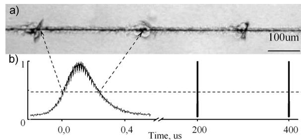
Figure 1. The damage track in optical fiber under the laser pulse train: a) the micrograph of the damaged F1, b) the temporal dependence of the laser intensity (in arbitrary units). The laser radiation propagated from right to left.
