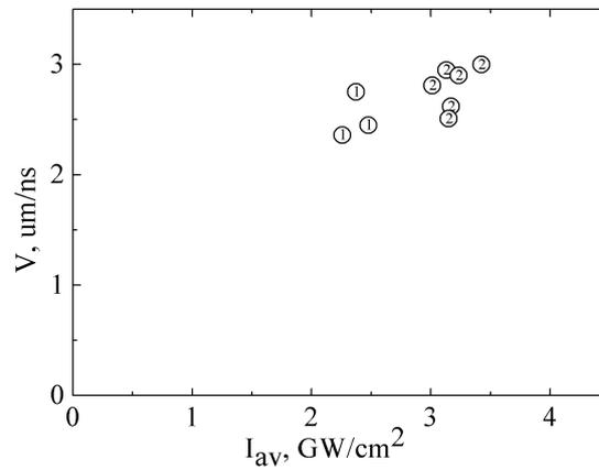
Figure 4. The dependence of the LSD velocity vs. the average laser intensity during LSD.
