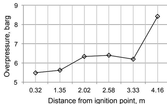
Figure 4: Acetylene/air explosion at for stoichiometric concentration
