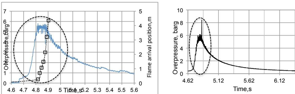
Figure 3 : Smoothing pressure-time histories (based on P1, 0.32 m from ignition point) and flame arrival time for stoichiometric premixed  $C_2H_2$ /air in straight pipe (left). Right is the actual graph.
