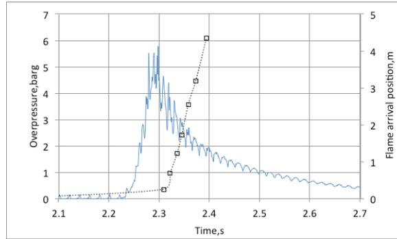
Figure 2: Pressure-time history (P1 based) and flame arrival time for stoichiometric premixed  $H_2$ /air in straight pipe.
