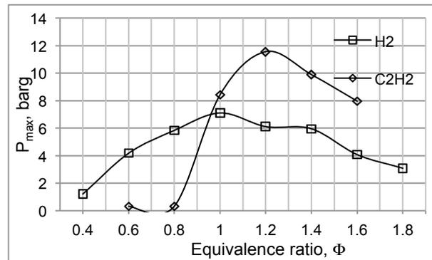
Figure 5: Maximum pressure at various equivalence ratio of hydrogen/air and acetylene/air mixture
