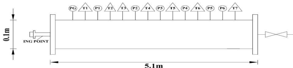
Figure 1 Explosion test rig
