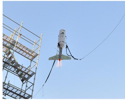
**Fig. 4.** PDRE flight system model Todoroki II [29, 30]
