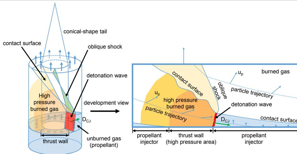
Fig. 5. Schematics of rotating detonation engine
