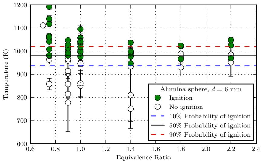
Figure 4: Hot particle ignition temperature as a function of equivalence ratio at atmospheric temperature and pressure
