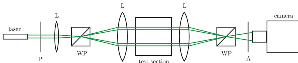
Figure 2: Shearing interferometer schematic (P: polarizer, L: lens, WP: Wollaston prism, A: analyzer)
