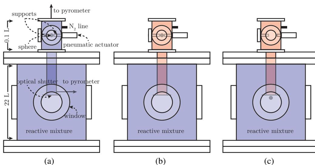
Figure 1: Experimental procedure for igniting a reactive mixture using a moving hot sphere, reactive mixture is shown in blue and N<sub>2</sub> is shown in red
