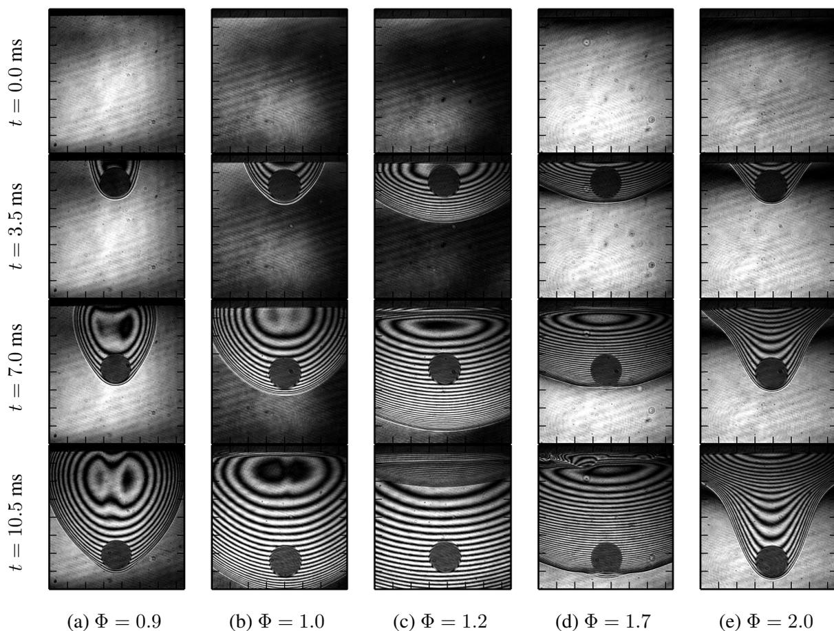
Figure 5: Flame propagation in *n*-hexane-air at various equivalence ratios and an initial temperature and pressure of 298 K and 100 kPa, respectively
