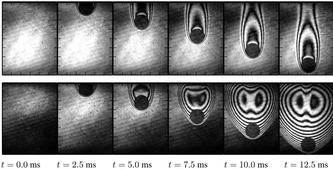
Figure 3: Infinite fringe interferometer images of a no ignition (top) and ignition (bottom) events with sphere temperatures of  $979\text{ K} \pm 27\text{ K}$  and  $981\text{ K} \pm 1\text{ K}$ , respectively, in *n*-hexane-air with an equivalence ratio of 0.9
