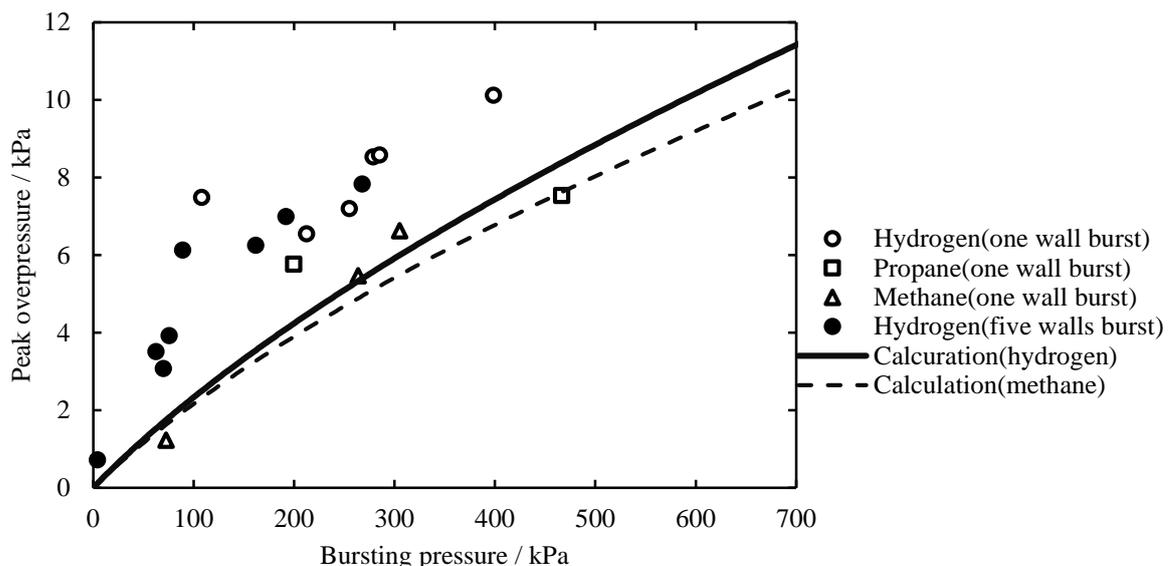
Figure 3, Relation between the bursting pressure and first peak overpressure at 5 m away from vessel center. The curve represents calculated values of vessel bursting by high pressure without combustion reaction.
