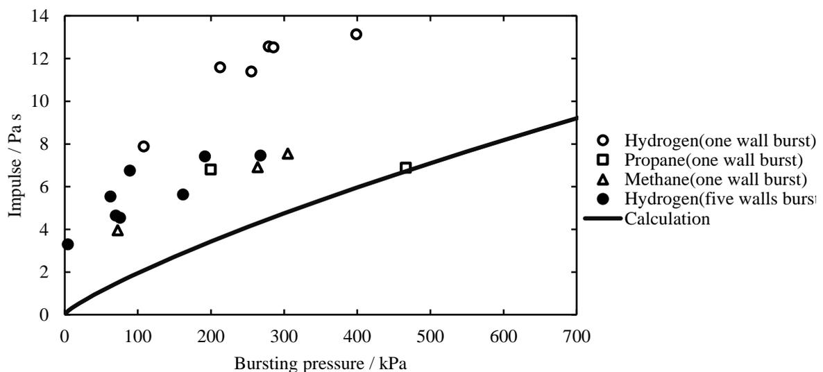
Figure 4, Relation between bursting pressure and impulse at 5 m away from vessel center. The curve represents calculated values of vessel bursting by high pressure mixtures of hydrogen-air.
