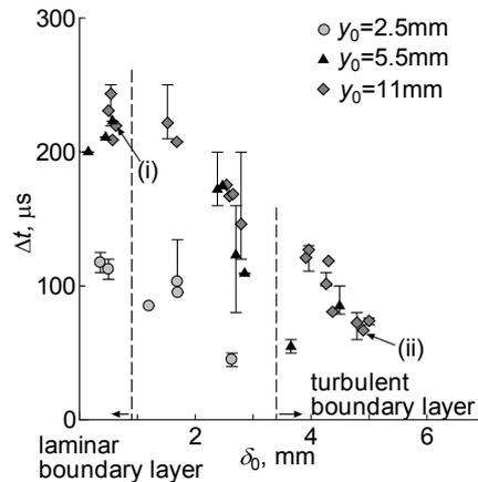
Figure 4. Required time for detonation initiation versus the boundary layer thickness in the case of forced ignition outside the boundary layer for  $M_s$  of 2.1.
