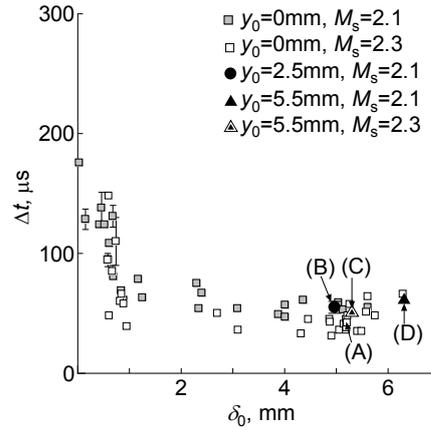
Figure 2. Required time for detonation initiation versus the boundary layer thickness in the case of forced ignition inside the boundary layer.
