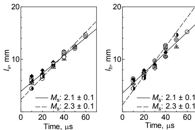
Figure 6. History of flame kernel size for  $y_0$  of 11 mm before contacting to neither the boundary layer nor the walls.  $l_v$ : vertical length of the flame kernel.  $l_h$ : horizontal length of the flame kernel.
