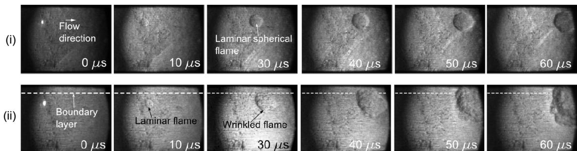
Figure 5. Propagating flame in the case of forced ignition outside the boundary layer. (i) and (ii) correspond to them in Fig. 4. (i)  $y_0 = 11 \text{ mm}$ ,  $M_s = 2.2$ ,  $\delta_0 = 0.6 \text{ mm}$  (The boundary layer cannot be seen in the images.), (ii)  $y_0 = 11 \text{ mm}$ ,  $M_s = 2.1$ ,  $\delta_0 = 4.9 \text{ mm}$ .
