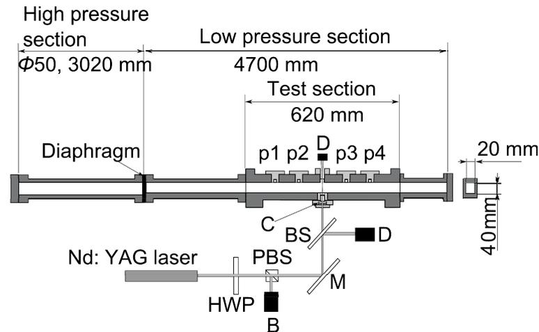
Figure 1. Schematic figure of shock tube and laser ignition system. HWP: half wave plate, B: beam stopper, PBS: polarizing beam splitter, M: mirror, BS: beam splitter, C: condensing lens, D: laser power detector.
