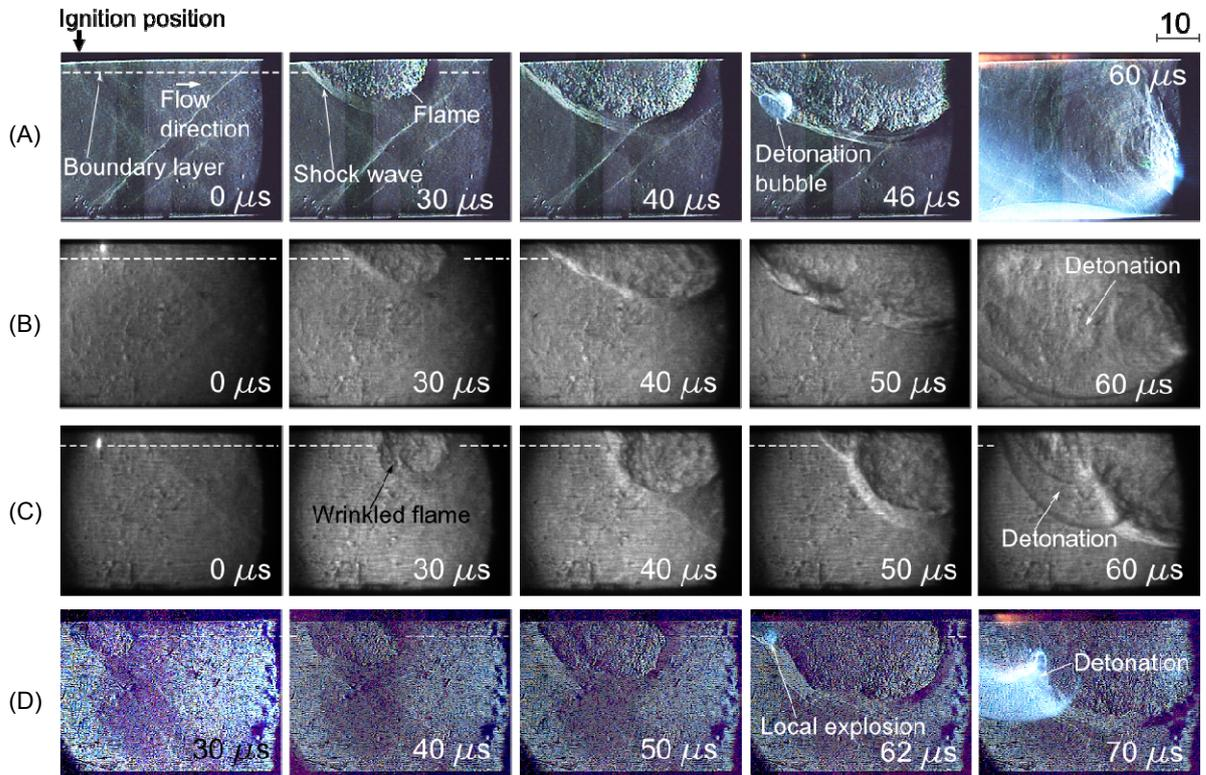
Figure 3. Propagating flame and detonation initiation in the case of forced ignition inside the boundary layer. (A) - (D) correspond to them in Fig. 2. (A)  $y_0 = 0$  mm,  $M_s = 2.4$ ,  $\delta_0 = 5.2$  mm, (B)  $y_0 = 2.5$  mm,  $M_s = 2.2$ ,  $\delta_0 = 5.0$  mm, (C)  $y_0 = 5.5$  mm,  $M_s = 2.2$ ,  $\delta_0 = 5.0$  mm, (D)  $y_0 = 5.5$  mm,  $M_s = 2.0$ ,  $\delta_0 = 6.3$  mm.
