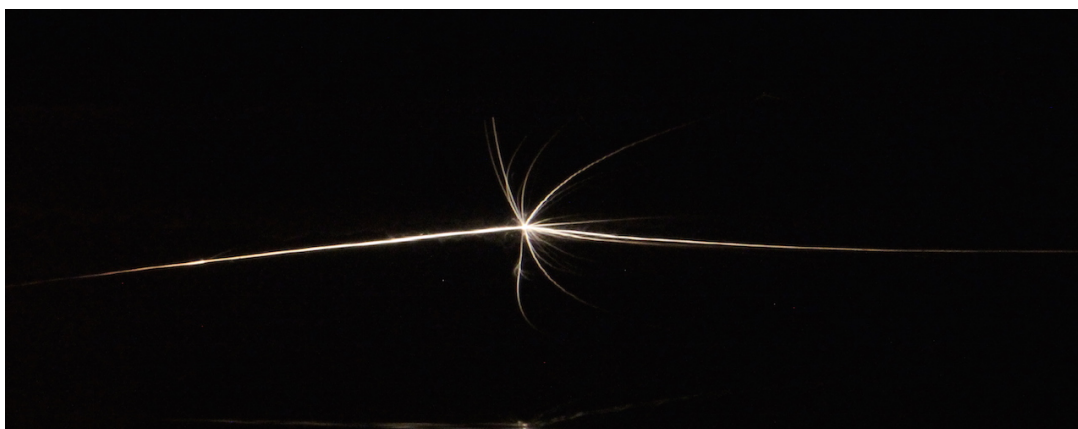
Figure 4: Long exposure photograph of iron particle exploding in oxygen/argon environment
