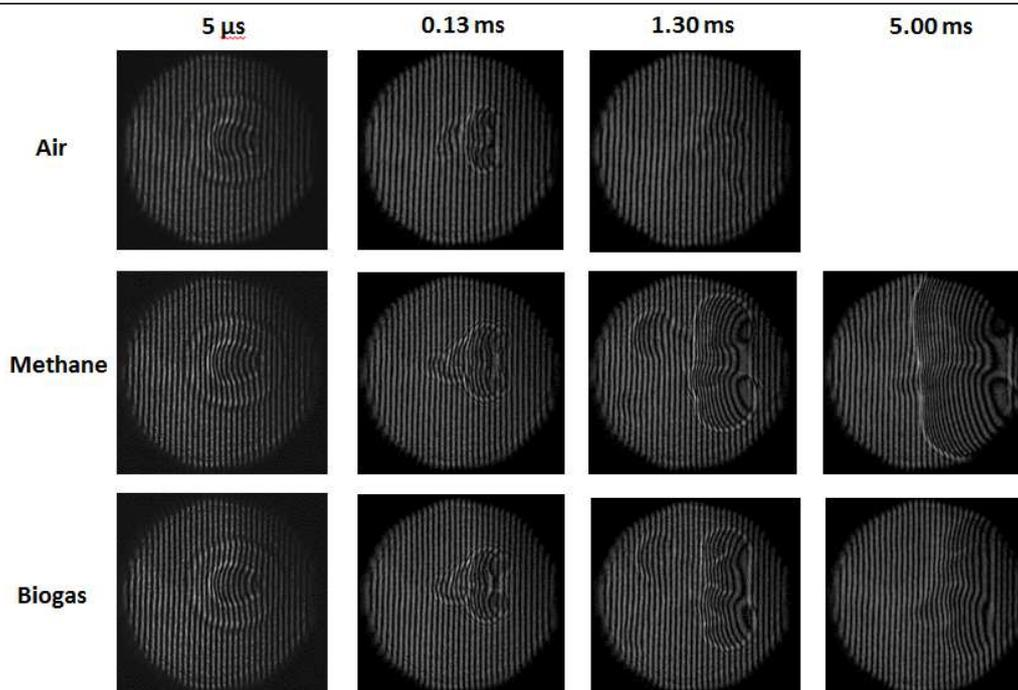
Figure 6: Interferometer images of breakdown in air, ignition of methane ( $\phi = 0.6$ ), and ignition of biogas ( $\phi = 0.6$ ), at an incident energy of 21.5 mJ and  $T = 298$  K,  $p = 1$  atm.
