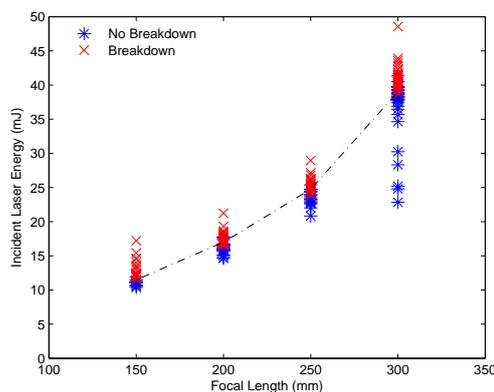
Figure 2: Breakdown threshold for 150, 200, 250, and 300 mm focal lengths in air at 1 atm, 298 K.
