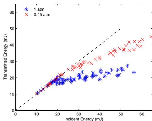
Figure 1: Transmitted versus incident energy at 0.45 atm and 1 atm and 298 K.
