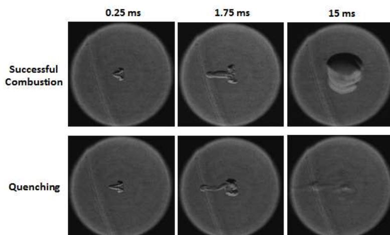
Figure 5: Schlieren images of quenched flame and ignition of biogas mixture,  $\phi = 0.65$ , with incident energies 27.5 mJ and 28 mJ, respectively.
