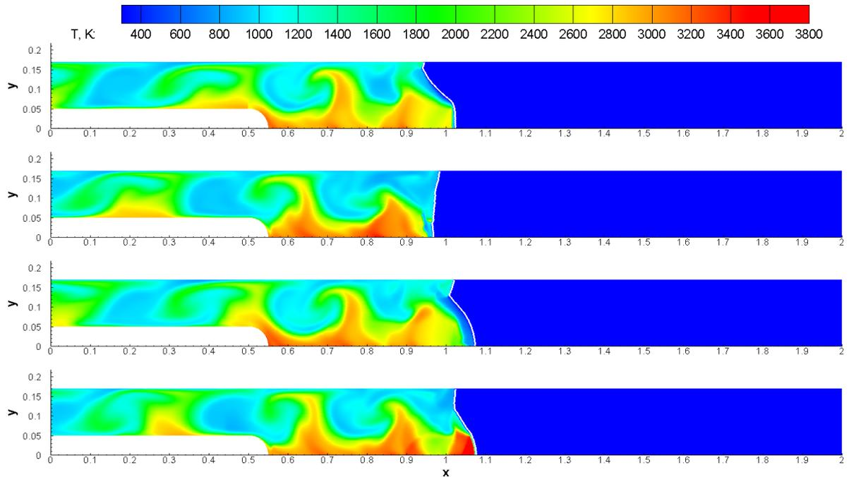
Fig. 2. Phases of galloping layered detonation in a channel with bench (temperature fields).
