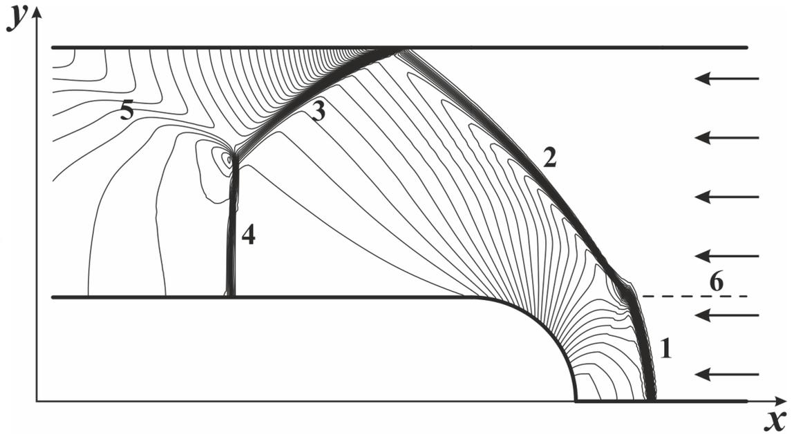
Fig. 1. Stationary detonation in the combustible mixture layer (temperature isolines).
