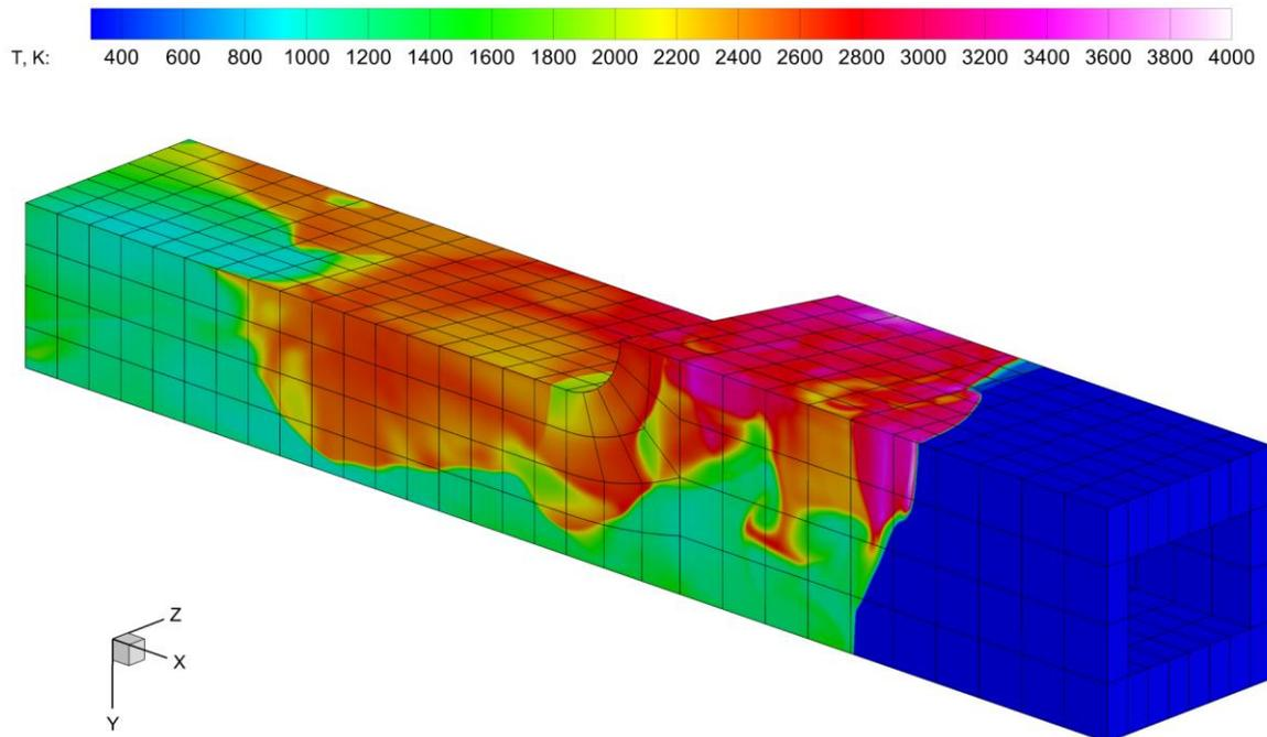
Fig. 7. Temperature field under 3D galloping layered detonation in a channel with inclined bench. The layer is located near the upper wall.
