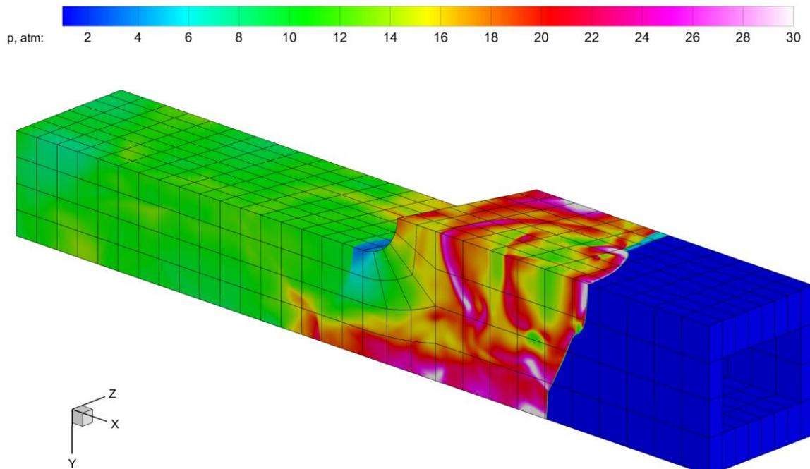
Fig. 6. Pressure field under 3D galloping layered detonation in a channel with inclined bench. The layer is located near the upper wall.
