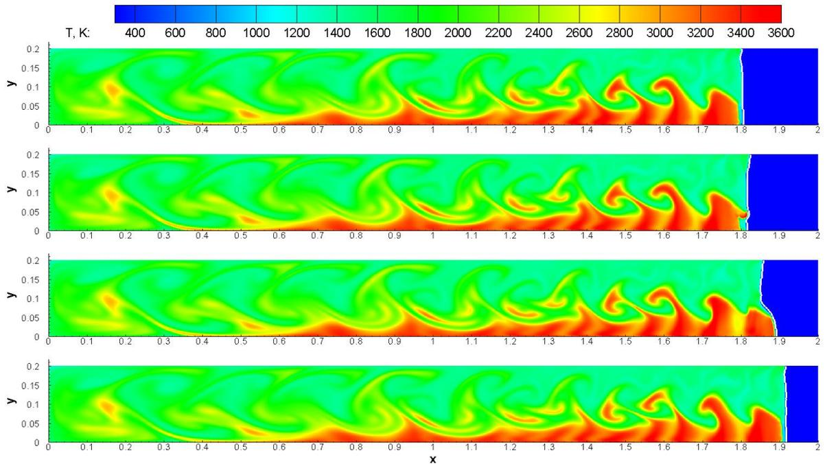
Fig. 3. Phases of galloping layered detonation in a channel with blocking wall (temperature fields).
