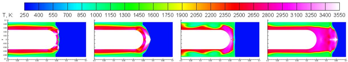
Fig. 4. Galloping layered detonation in a circular channel with a rod in the center.
