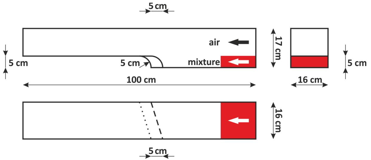
Fig. 5. Three projections of the 3D channel with sizes, air and mixture jet shown.
